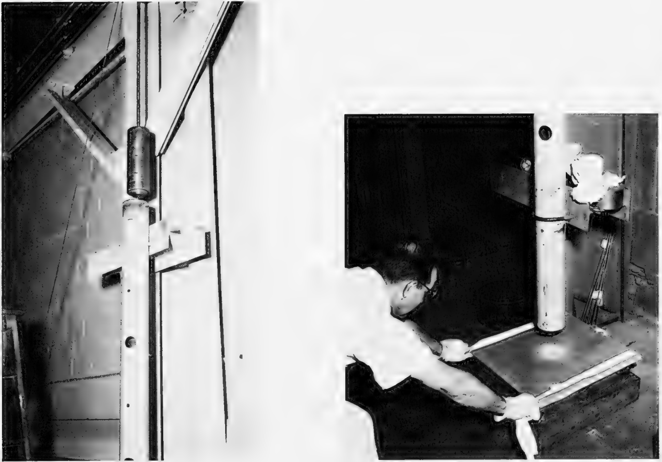
a. Impactor at Top of 20 Ft. Long Seamless Steel Tube b. Panel Under Test on Supporting Frame
