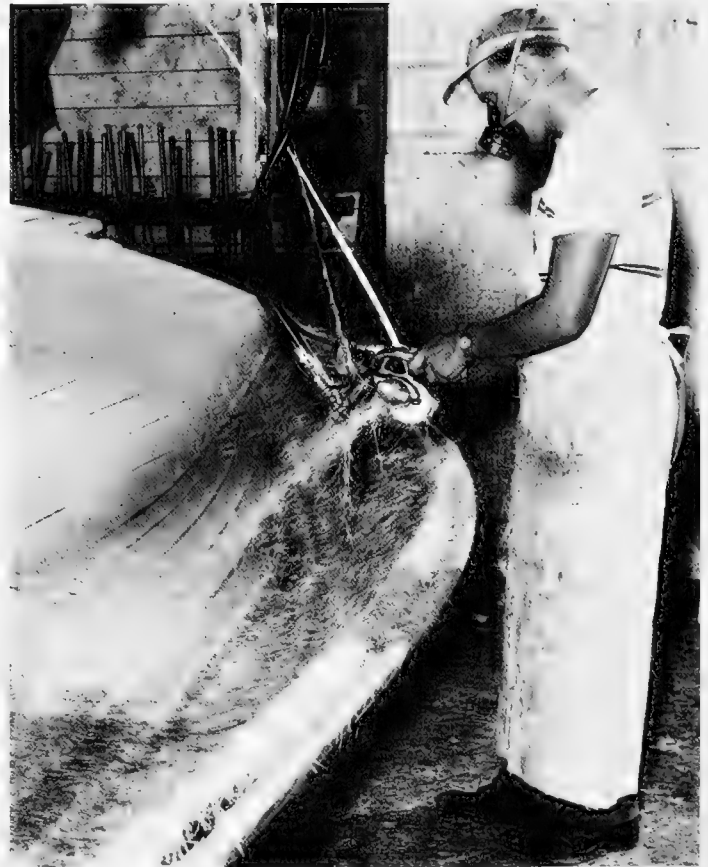
Fig. 4-23. Spray gun depositing chopped fibers and resin on hull mold (Courtesy Larsen Boat Company)
