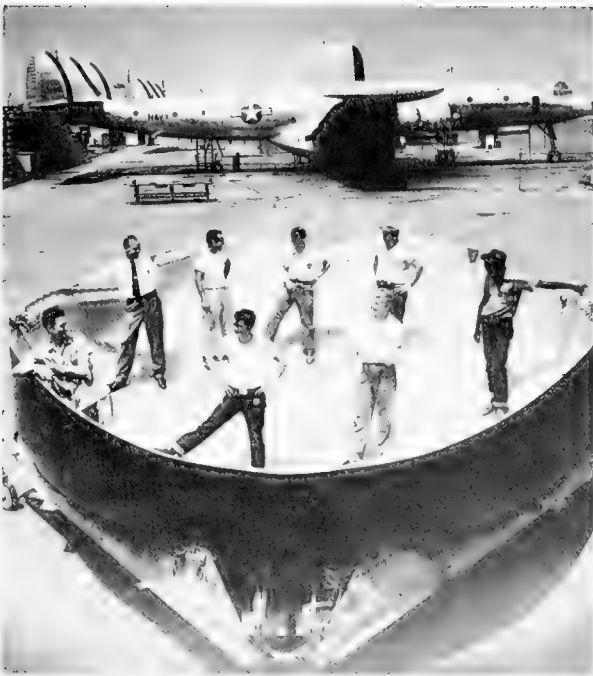
Fig. 1-1. Largest Aircraft Radome, 29' Long, 20' Wide and 7' Deep (Courtesy Zenith Plastics Company, Division of Minnesota Mining and Manufacturing Company)
