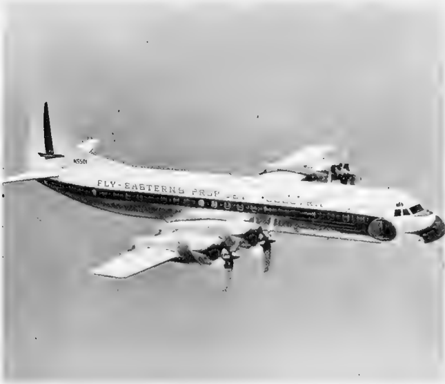
Fig. 1-18. Passenger Aircraft with many Fiberglass Parts; Wing Tips, Tail Cone, Seats, Coat Racks, Window Frames, Bulkheads, etc. (Courtesy Lockheed Aircraft Corporation)
