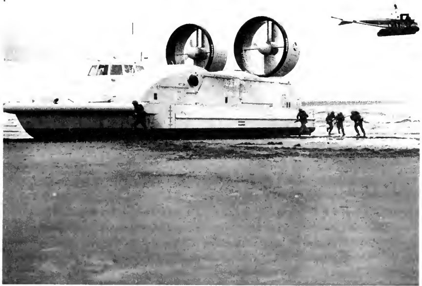
The Navy's Hydroskimmer (SKMR-1) is being used as a research and operational test vehicle. Built by Bell Aerospace the 35-ton craft is the largest air-cushion vehicle constructed in the United States.
