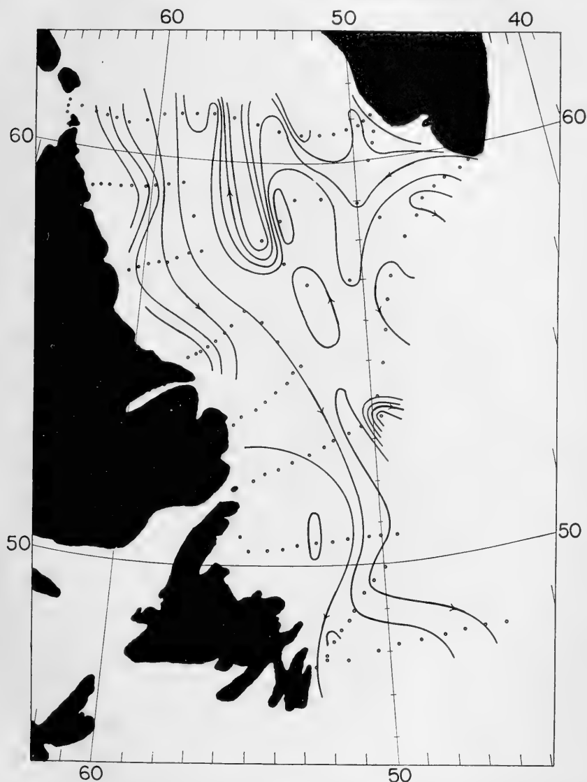
FIGURE 4.—An example of a transport map, each line representing a volume of current of 1,000,000 cubic meters per second. Based on General Greene's survey July 4–August 8, 1931.
