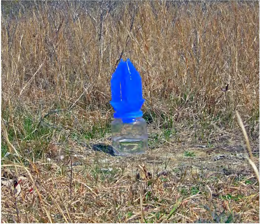
Figure 1. Vane Trap. Unscented, semi-transparent, fluorescent blue vane trap, type BVT1, from SpringStar ® LLC showing the clear plastic collecting jar with a screw-on plastic lid to hold the blue UV-reflective vanes. (Photographed by Richard L. Orr)
