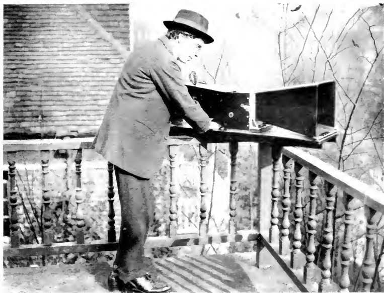
PROFESSOR A. M. LOW, WITH THE AUDIOMETER WHICH HE INVENTED TO PHOTOGRAPH NOISE
