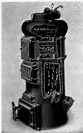
FIG. 38. Heating plant showing safety valve.
