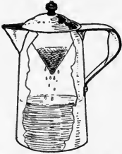
FIG. 117. Drip funnel in percolator.
