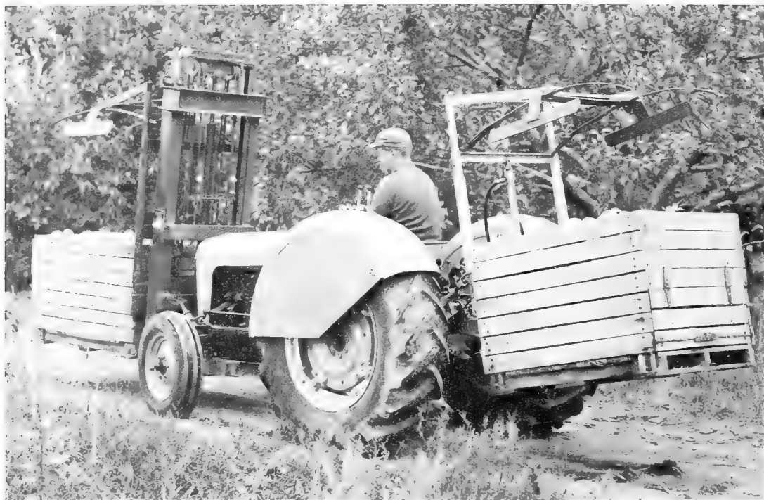
Figure 3.—Tractor equipped with forklift attachments being used to carry apples out of an orchard. Other types of lift equipment are available.
