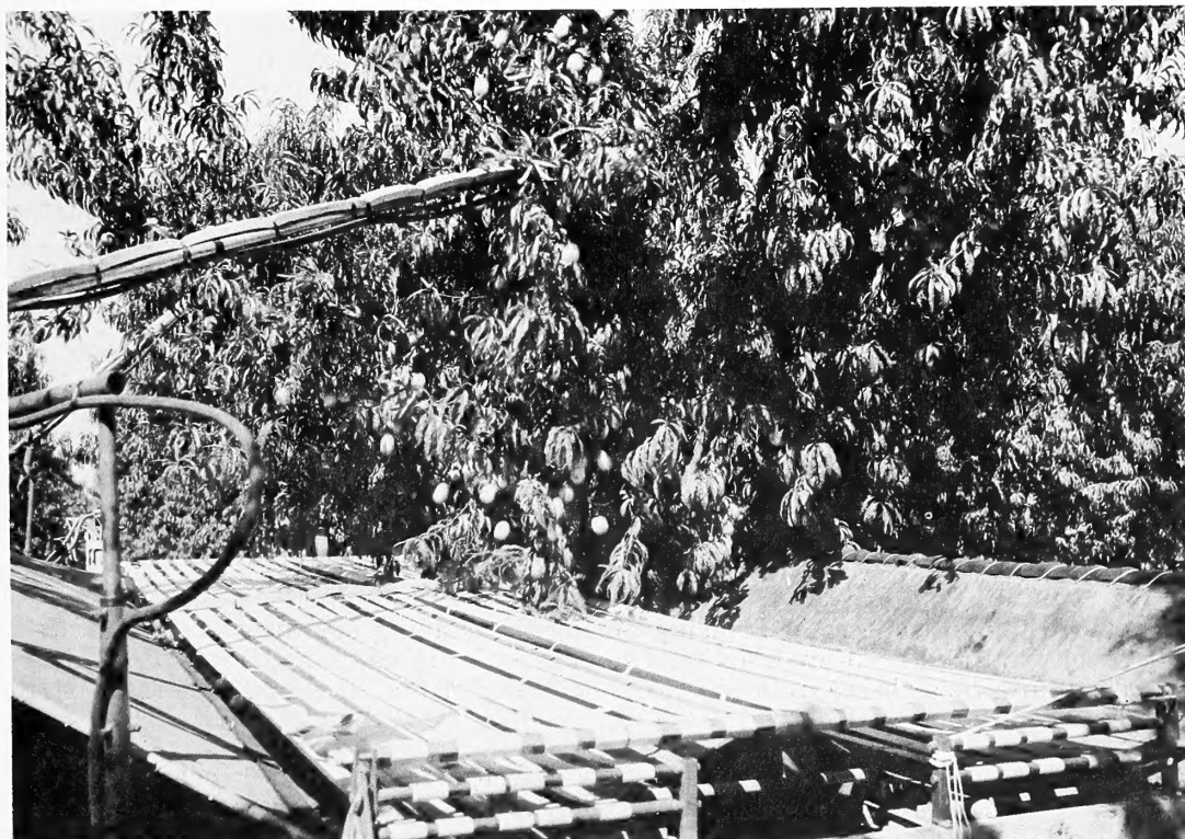
Figure 1.—Boom shaker and catching frame are being used to experimentally harvest peaches. Note parallel layers of decelerator strips. These slow the descent of the falling peaches and keep the peaches from bruising when they strike the catching frame.
