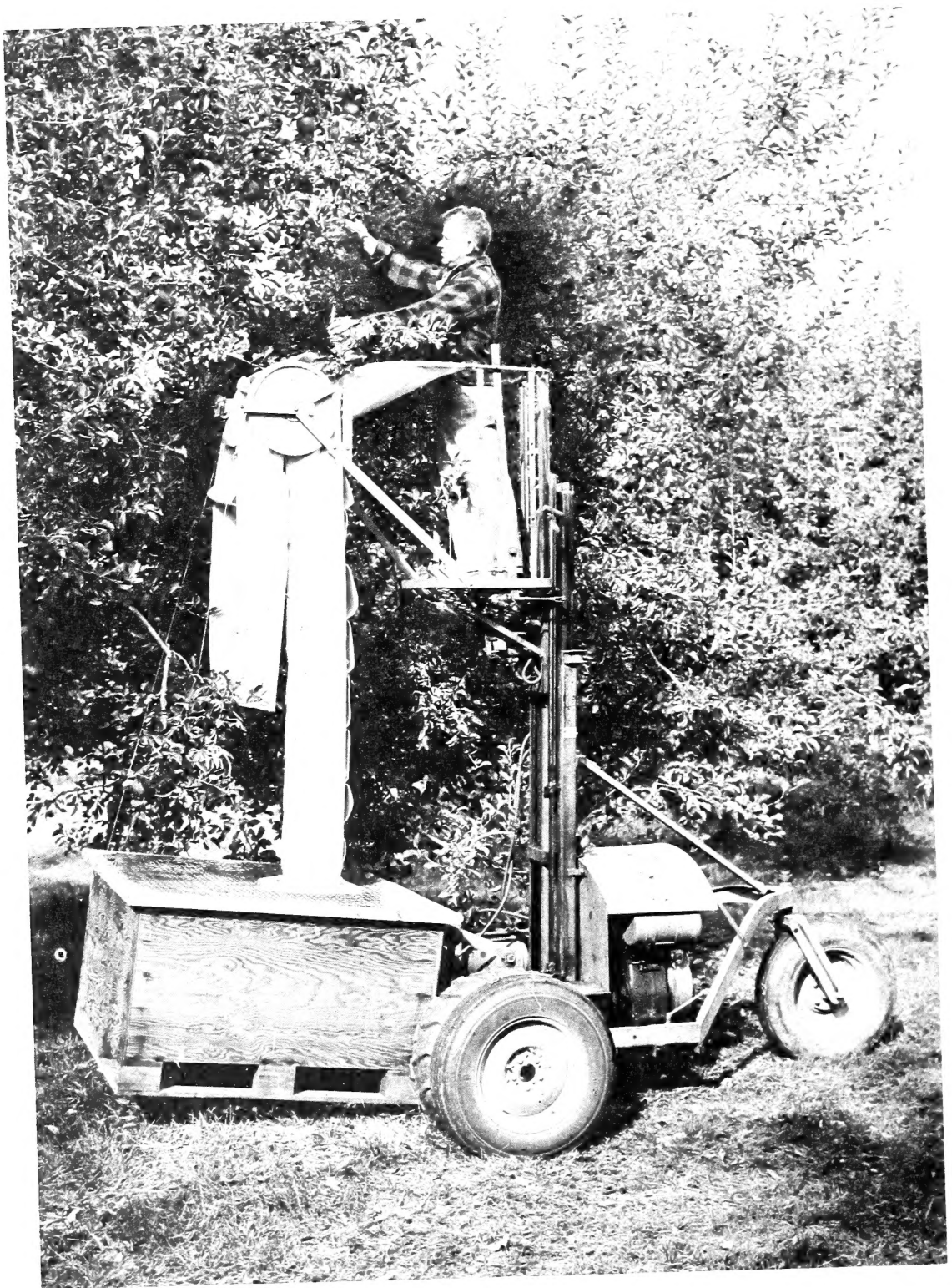
Figure 2.—Worker is utilizing a self-propelled platform with pick-and-drop equipment to pick apples.
