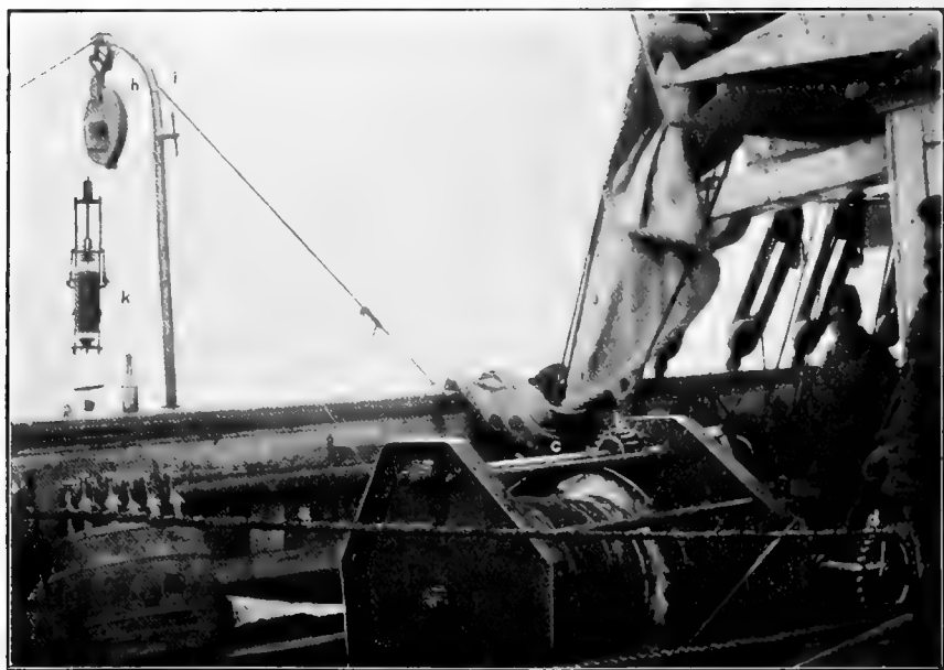
Fig. 3. Winch for soundings and hydrographical work; C. B. Thostrup phot. a—e , see above (Fig. 2). h , meter-wheel. i , davit. k , water-bottle.
