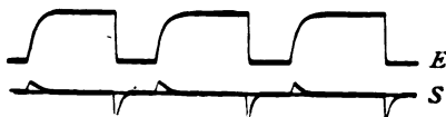
1.—Curves showing the variations of current in the exciting circuit and in the secondary circuit of a medical coil. The growth and rupture of the exciting circuit are seen above, and the corresponding currents in the secondary circuit are below.
