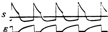
3.—The same coil with core, and rapid interruptions showing interference of the long waves of the secondary circuit.
