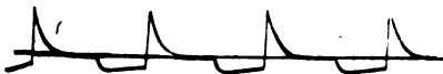
7.—As fig. 6, but with secondary coil three times as long, showing longer duration of the wave at break.
