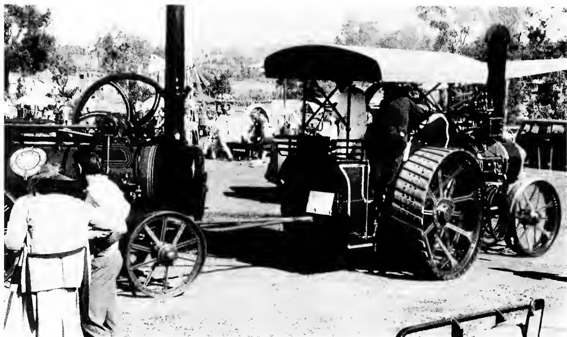
FIG. 7. The Museum's fully restored Garrett steam traction engine and its portable Ransomes, Sims and Jefferies steam engine at an antique machinery show.
