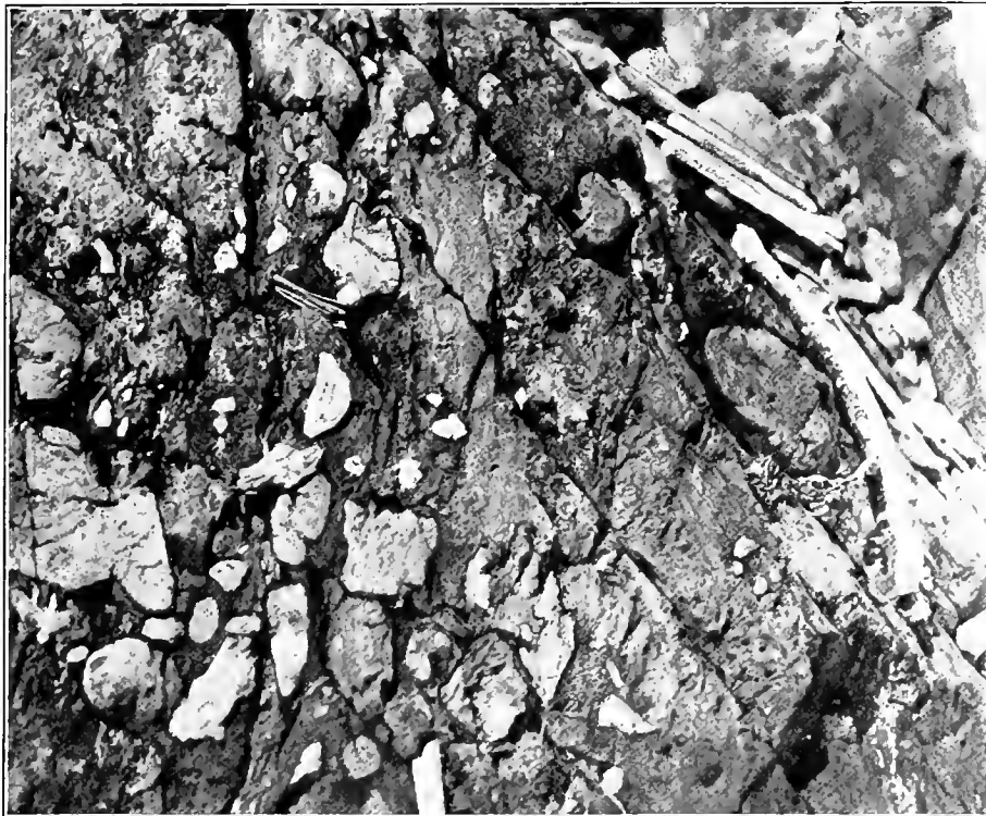
11. BRECCIATED BAND OF MASSIVE FINE-GRAINED GREENSTONE AT UPPER TWIN FALLS. The fragments are mainly dense, light-colored greenstone. The matrix is a schistose, chloritized greenstone containing streaks of chlorite.
