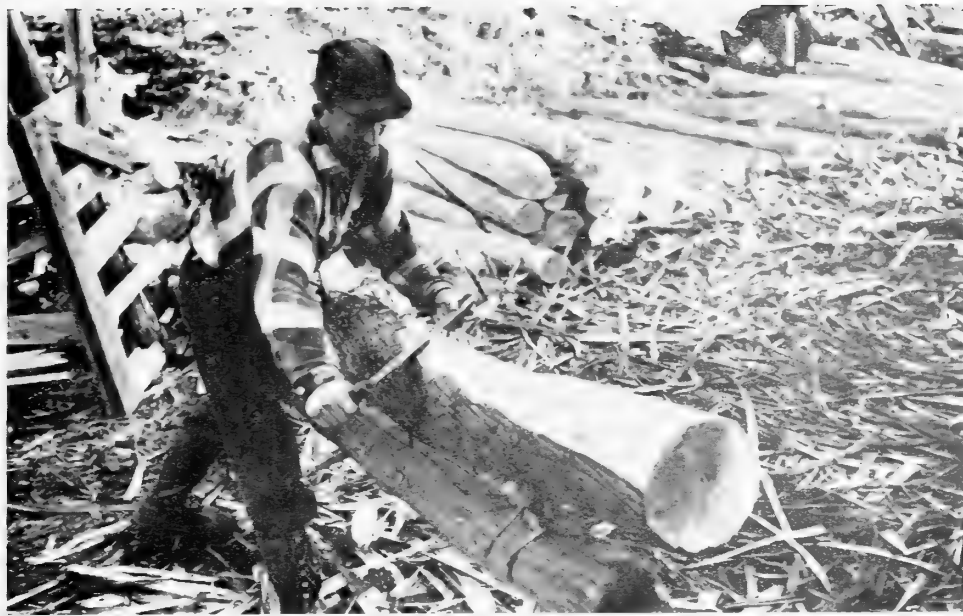
FIGURE 16.— Cedar fence post being "peeled" in Upper Michigan. Cedar posts valued in excess of $2,000,000 were produced in 1954.
