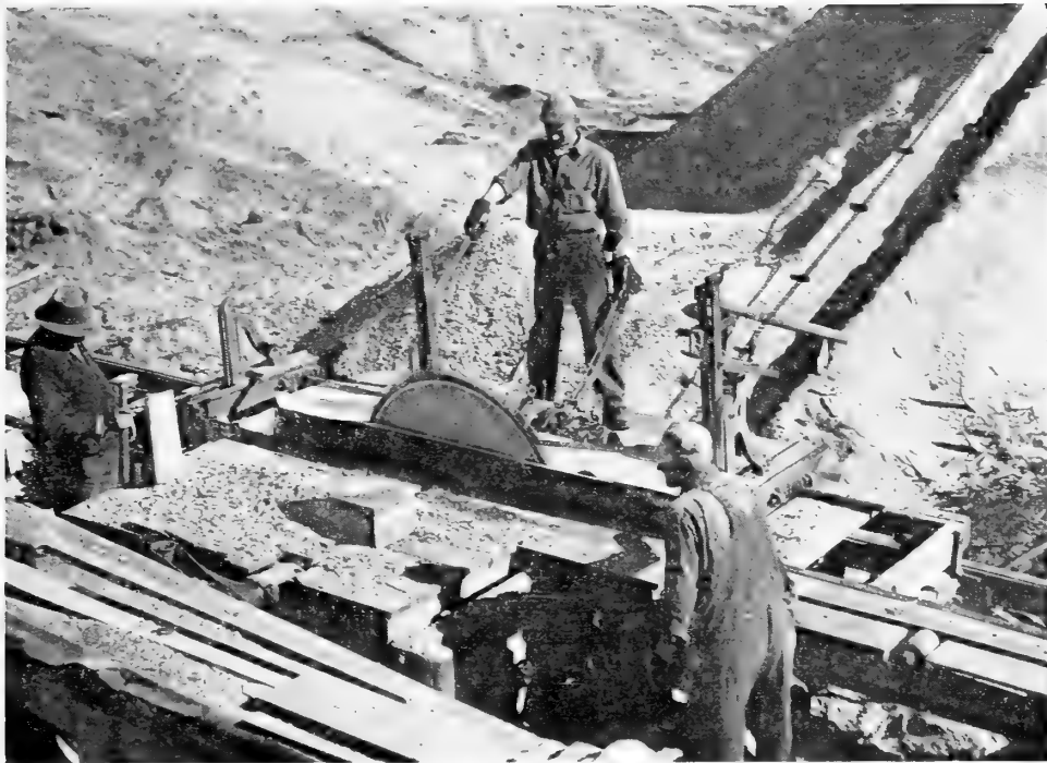
FIGURE 23.— Small sawmills account for about one-third of Michigan's lumber production. Because of misaligned or wornout equipment many small mills manufacture a poor grade of lumber. Much of it is miscut and unfit for commercial use. A recent lumber survey shows that about 35 percent of the small mill operators sawed for their own use, 40 percent operated on a custom basis, and only about 25 percent sawed for commercial markets.
