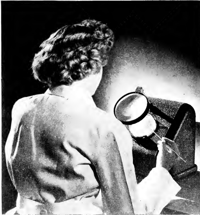
Fig. 29. Quebec colony counter in use. (Courtesy of the American Optical Company, Instrument Division, Buffalo, New York.)
