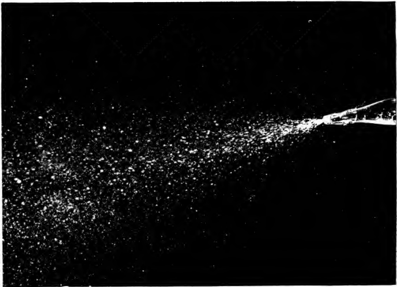
Fig. 44. Atomizing of droplets into the air by blowing out the last drop from a pipette. (From Johansson, K. R., and Ferris, D. H. Journal of Infectious Diseases , 1946, 78, 241.)
