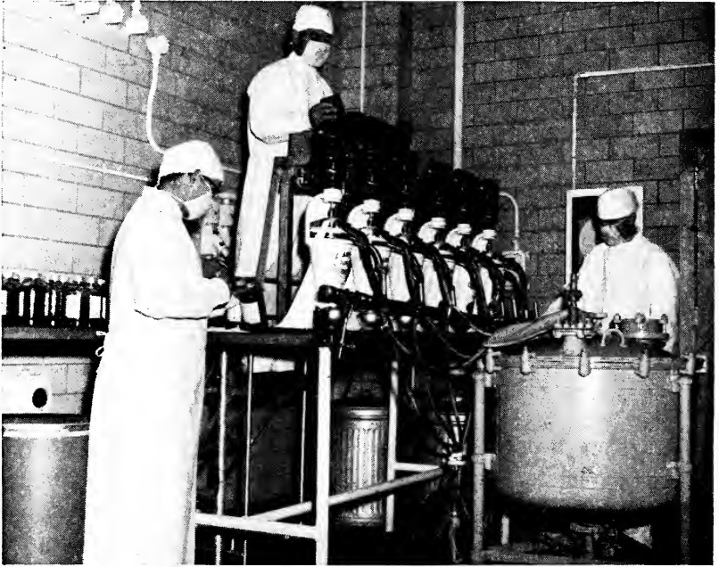
Fig. 57. Human blood fractionating laboratory. Poliomyelitis-Immune Globulin as well as Serum Albumin for the prevention of shock are separated from the blood after centrifuging. (Courtesy of Armour and Company, Chicago, Illinois.)
