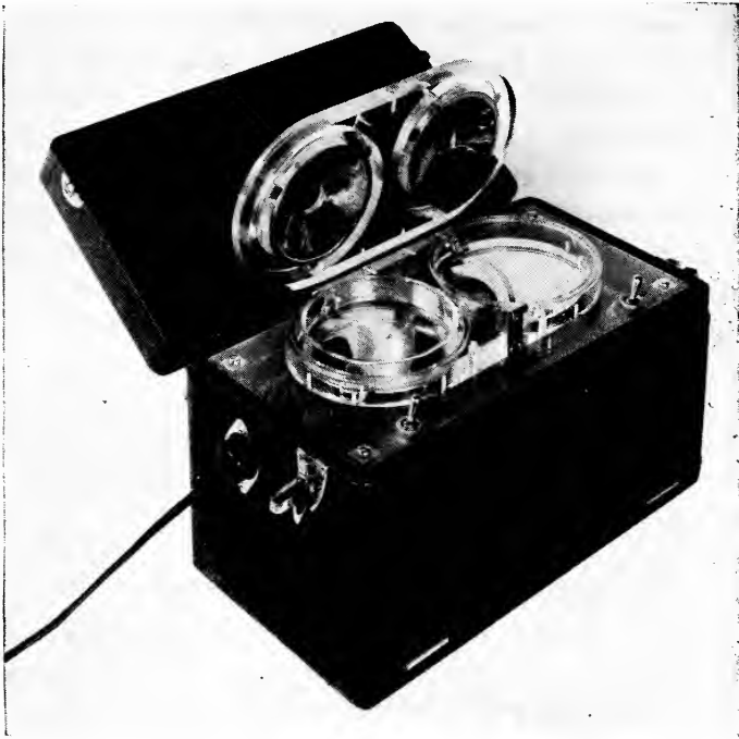
Fig. 42. Electrostatic air sampler showing exposed petri dishes. It employs a high voltage electrostatic field to precipitate organisms from a given volume of air into two specially prepared petri dishes. (Courtesy of the Lamp Division of General Electric Company, Schenectady, New York.)
