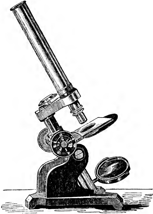
Field's "Society of Arts" Compound Microscope.
