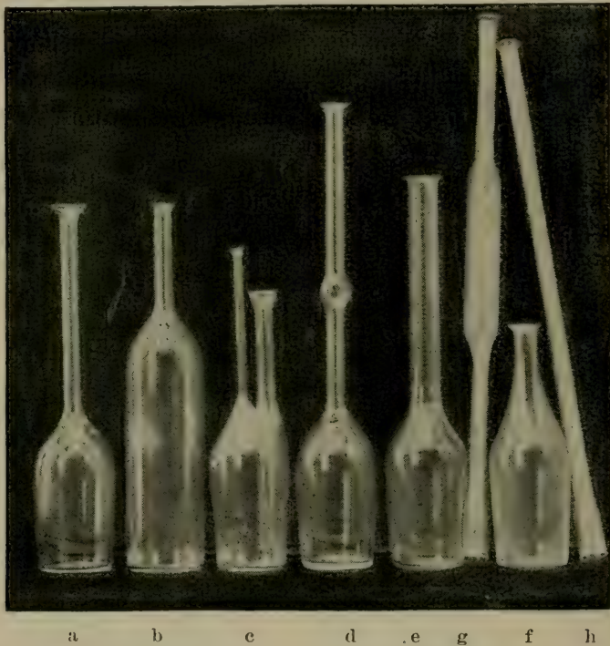
Fig. 5. Forms of Babcock test bottles; a , ordinary bottle for whole milk; b , bottle for skim milk, using double charge of milk; c , Ohlsson, or "B. & W." double-necked bottle for skim milk; d , e , bottles for testing cream; f , bottle with detachable neck; g , h , detachable necks for butter and cream.
