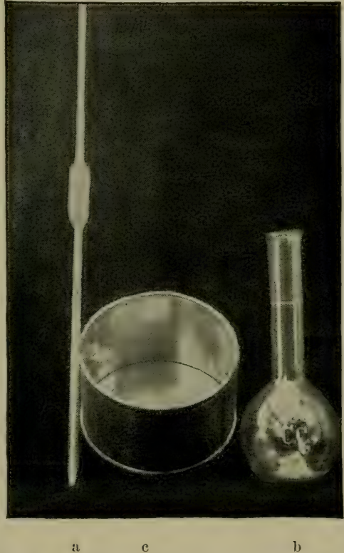
Fig. 23. Monrad rennet test. a , 5 c. c. pipette; b , 50 c. c. graduated flask; c , cup in which test is made.
