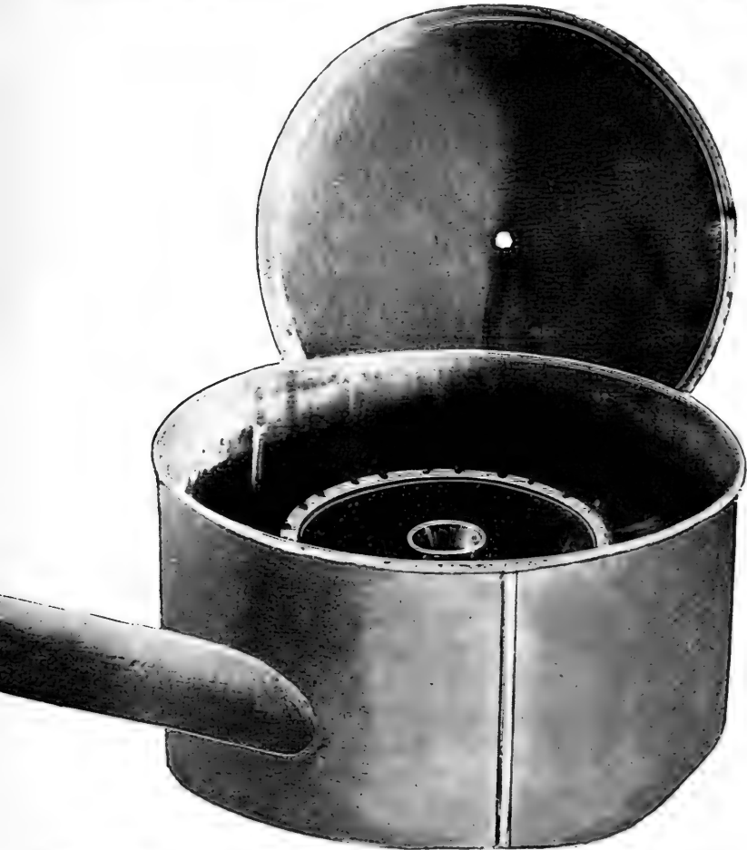
Fig. 4. Steam turbine centrifugal for Babcock test. (See opposite page.)
