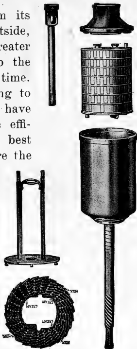
Fig. 26. Parts of United States separator bowl.
