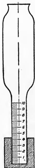
Fig. 66.—Casein tube and cork support. (Bull. 156, November, 1907, Univ. of Wis. Agri. Exp. Sta.)
