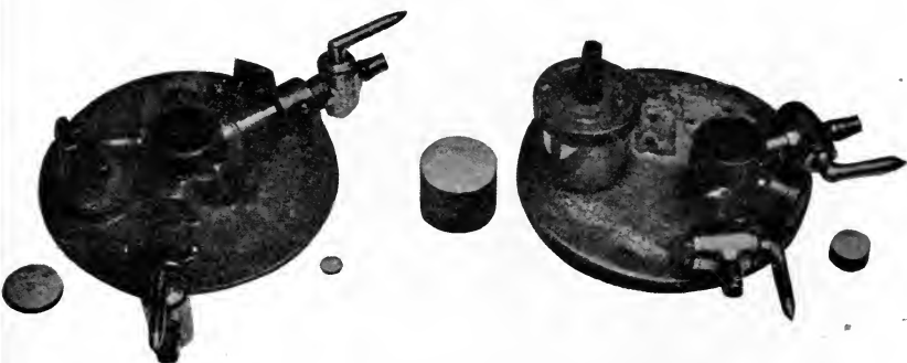
Fig. 130.—Two styles of pulsator head of Burrell-Lawrence-Kennedy machine. Blocks show sizes of filters. (Harding, Wilson, and Smith, Bull. No. 317, New York Agric. Exp. Sta.)
