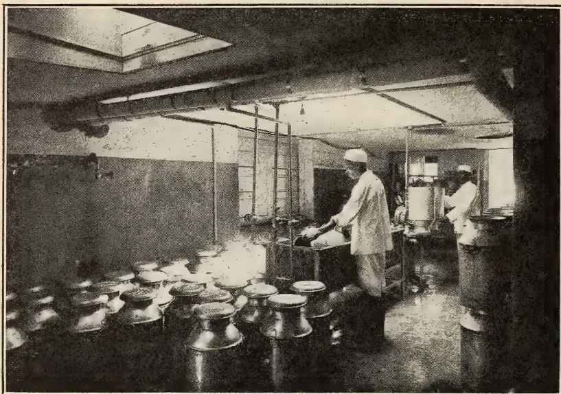
FIG. 21.—Washing, steaming, and drying cans.
