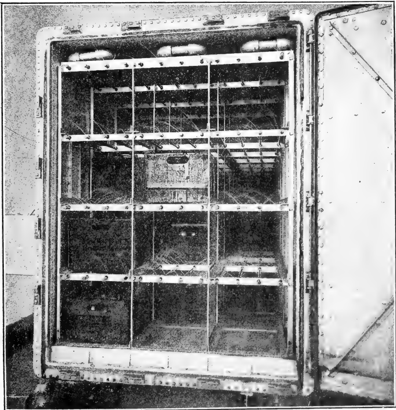
FIG. 12.—Front view of in-the-bottle pasteurizer, showing the fine sprays of hot water used in heating the milk.
