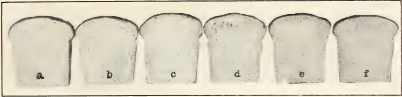
FIG. 1.—Loaves from clean wheat ( a ) and from wheat containing admixtures of rye: b , 1 per cent; c , 2 per cent; d , 3 per cent; e , 5 per cent; f , 10 per cent.
