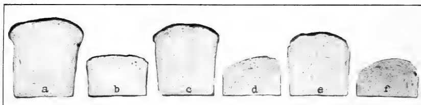
FIG. 2.—Effects of 10 per cent admixture of corn cockle in wheat: a , Patent flour (check); b , patent flour (10 per cent corn cockle); c , first-clear flour (check); d , first-clear flour (10 per cent corn cockle); e , second-clear flour (check); f , second-clear flour (10 per cent corn cockle).
