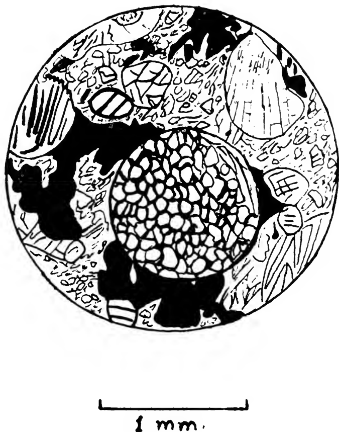
FIG. 7. Drawing of thin section of the chondrite Allegan illustrating typical silicate-metal relations.
