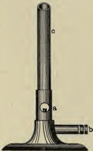
FIG. 525. — The Bunsen Burner.
