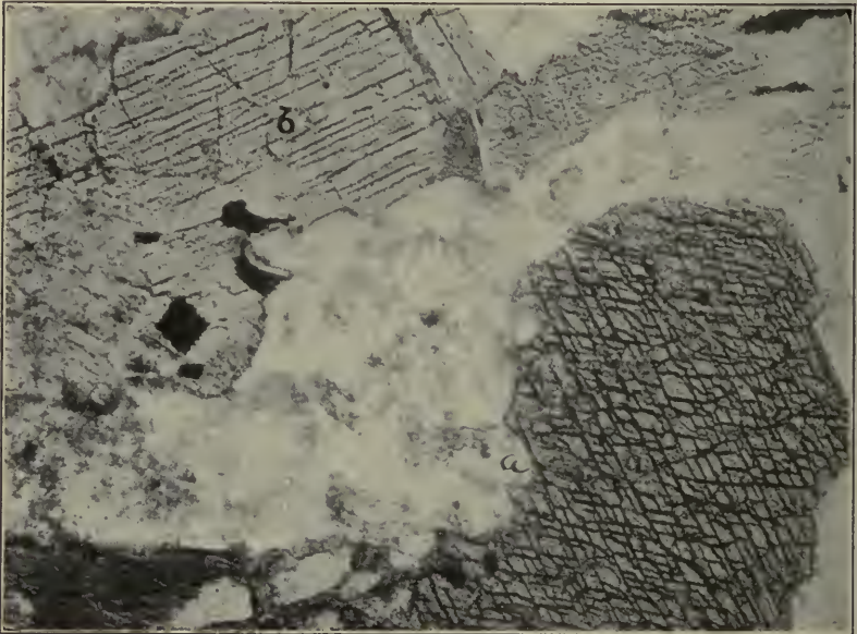
FIG. 478.—Section of Diorite, showing the Relief and Cleavage Angle, 124^{\circ} , of Hornblende a, and also the Parallel Cleavage b, when cut Parallel to the Vertical Axis.
