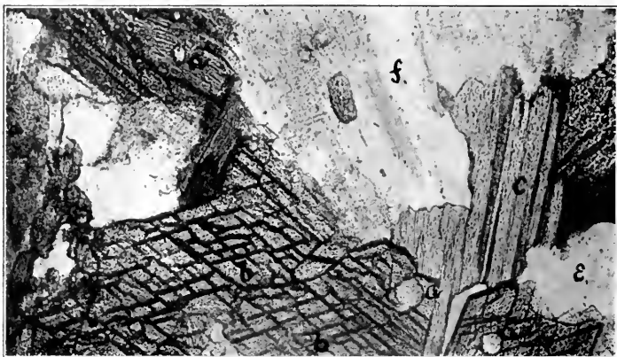
FIG. 515.—Section of a Mica-diorite, showing a , Apatite; b , Hornblende; c , Biotite; e , Quartz; and f , Feldspar partially Altered.
