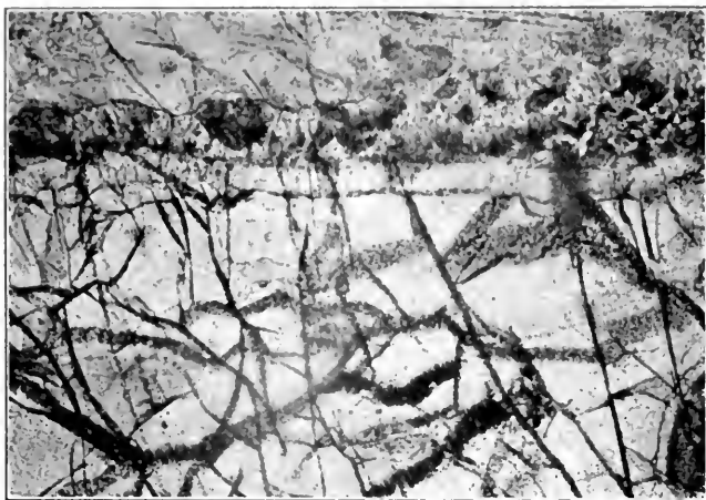
FIG. 487.—Section of Olivine, showing the Cracks filled with Secondary Magnetite and a Marginal Band of Enstatite and Hornblende.
