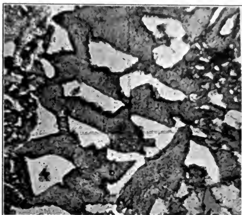
FIG. 427. — Enlarged Micropegmatite between Crossed Nicols. The Light Areas are Quartz, the Dark Orthoclase.
