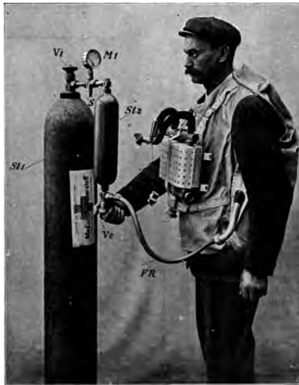
FIG. 19.—PNEUMATOGEN: II. TYPE: CHARGING THE BREATHING-BAG.
