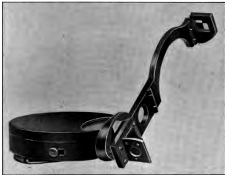
FIG. 4.—POCKET TRANSIT TAKING AN INCLINED BEARING.
