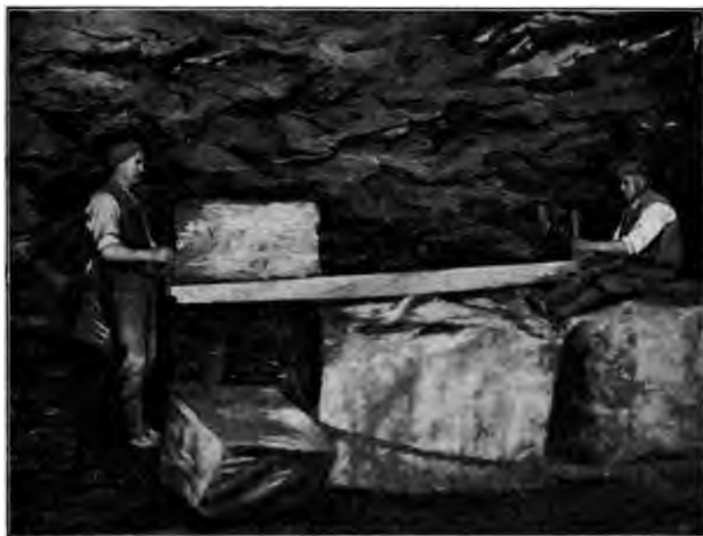
FIG. 12.—MEN SAWING AN ALABASTER-BLOCK IN FAULT MINE.
