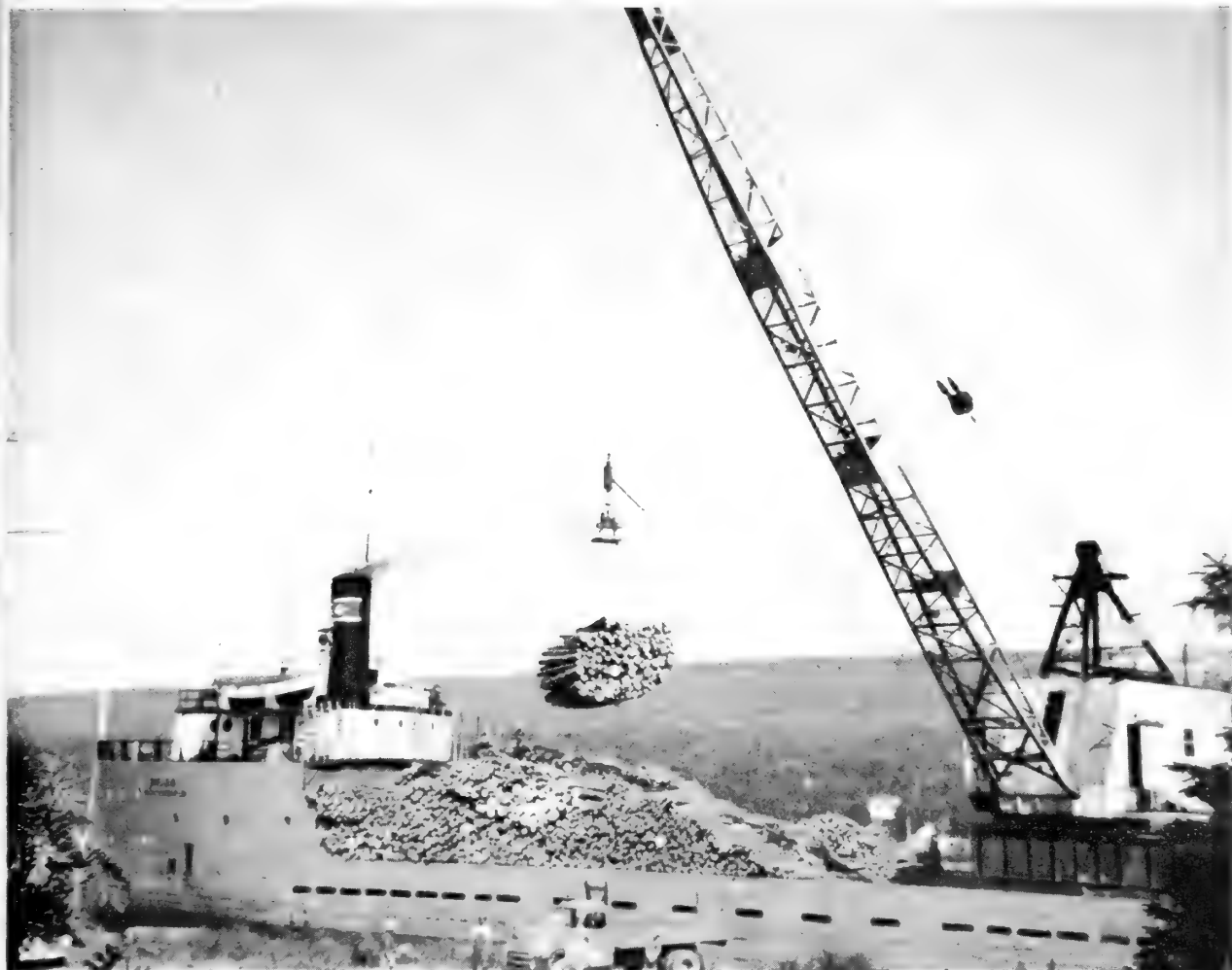
FIGURE 31.—Spruce and balsam pulpwood being loaded on Great Lakes freighter at Grand Marais, Minn. Fully loaded, the ship carries between 1,500 and 1,800 cords. The cargo is transported across Lake Superior to Munising, Mich., where it is unloaded and shipped by rail to Michigan and Wisconsin pulp and paper companies.
