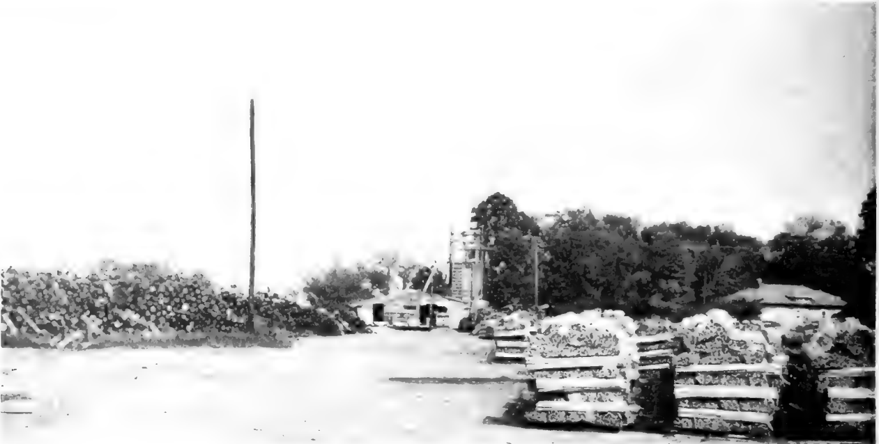
FIGURE 33.— The Wheeler Lumber Bridge & Supply Co. This mill manufactures lath almost entirely from aspen bolts. It is probably the largest mill of its kind in the State. Most of the lath produced in Minnesota is used for snow fences. (Photo courtesy Wheeler Lumber Bridge & Supply Co.)
