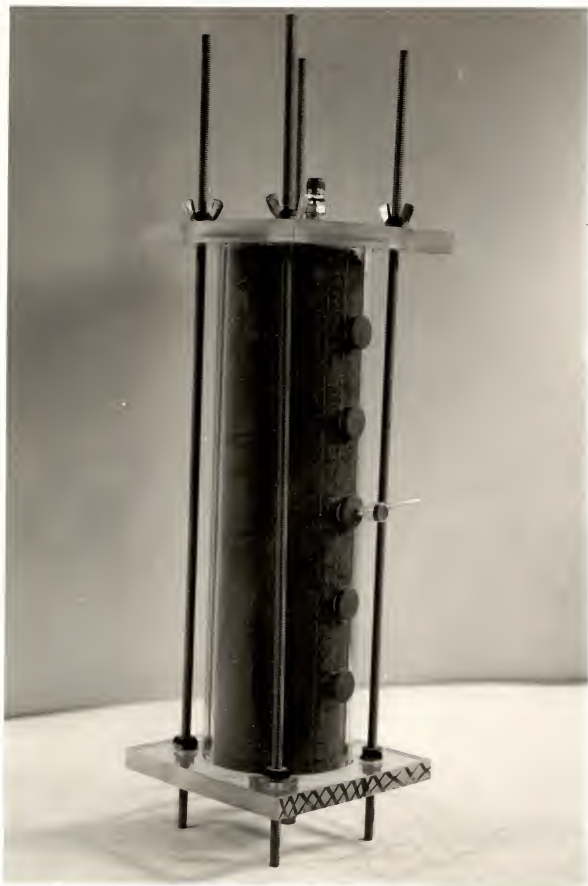
Figure 1. The general set-up of soil column during the displacement studies.
