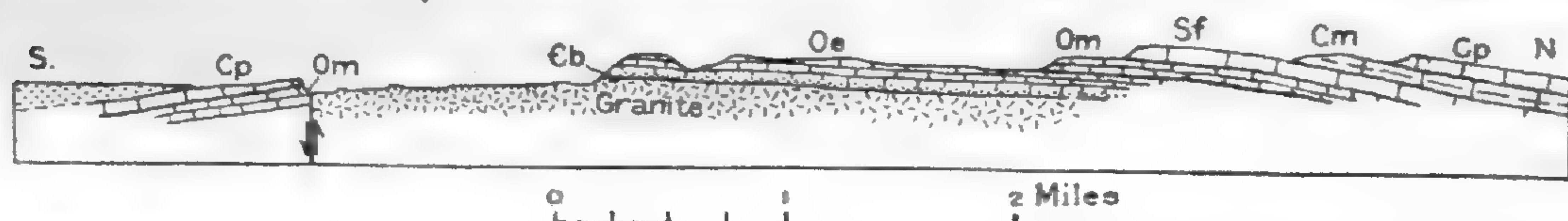
FIGURE 25.—Section through the south end of the Hueco Mountains, 20 miles north-northeast of Fabens, Tex. Cp, Limestone (Permian); Cm, limestone (Pennsylvanian and Mississippian); Sf, Fusselman limestone; Om, Montoya limestone; Oe, El Paso limestone; Eb, Bliss sandstone
