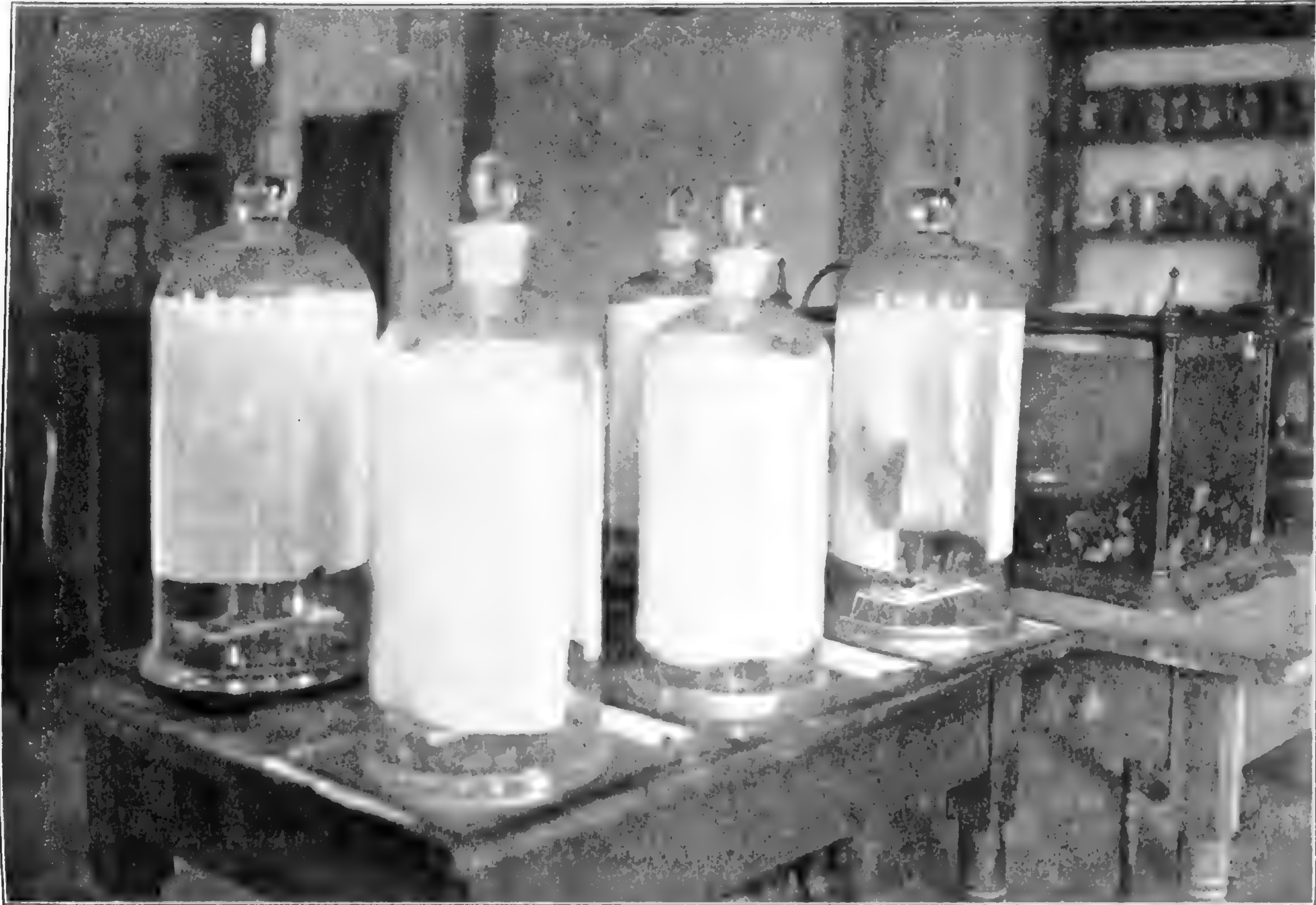
FIG. 1. —Bell jars in which the effect of hydrocyanic acid gas upon the germination of seeds is being determined.
