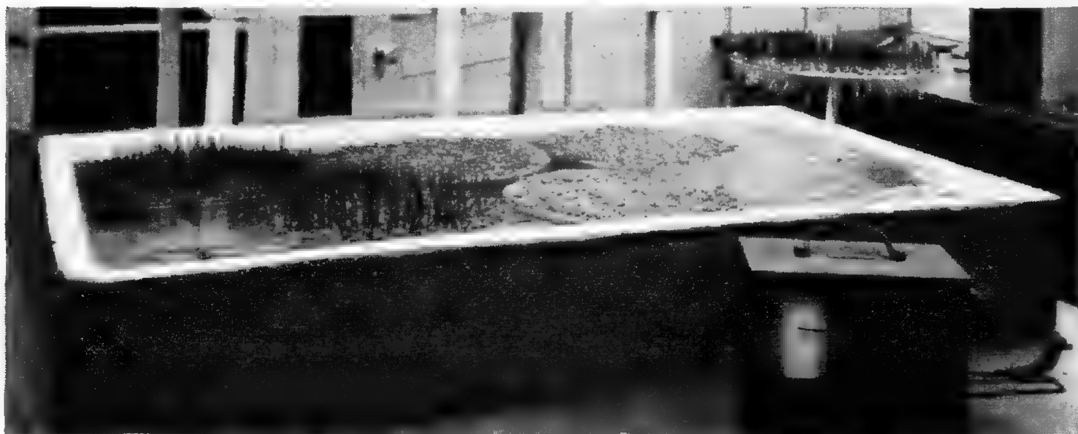
FIG. 2.—Method of germinating wheat seedlings on aluminum disks, which are floated in an enameled tank; disk to right elevated to show the plant roots.
