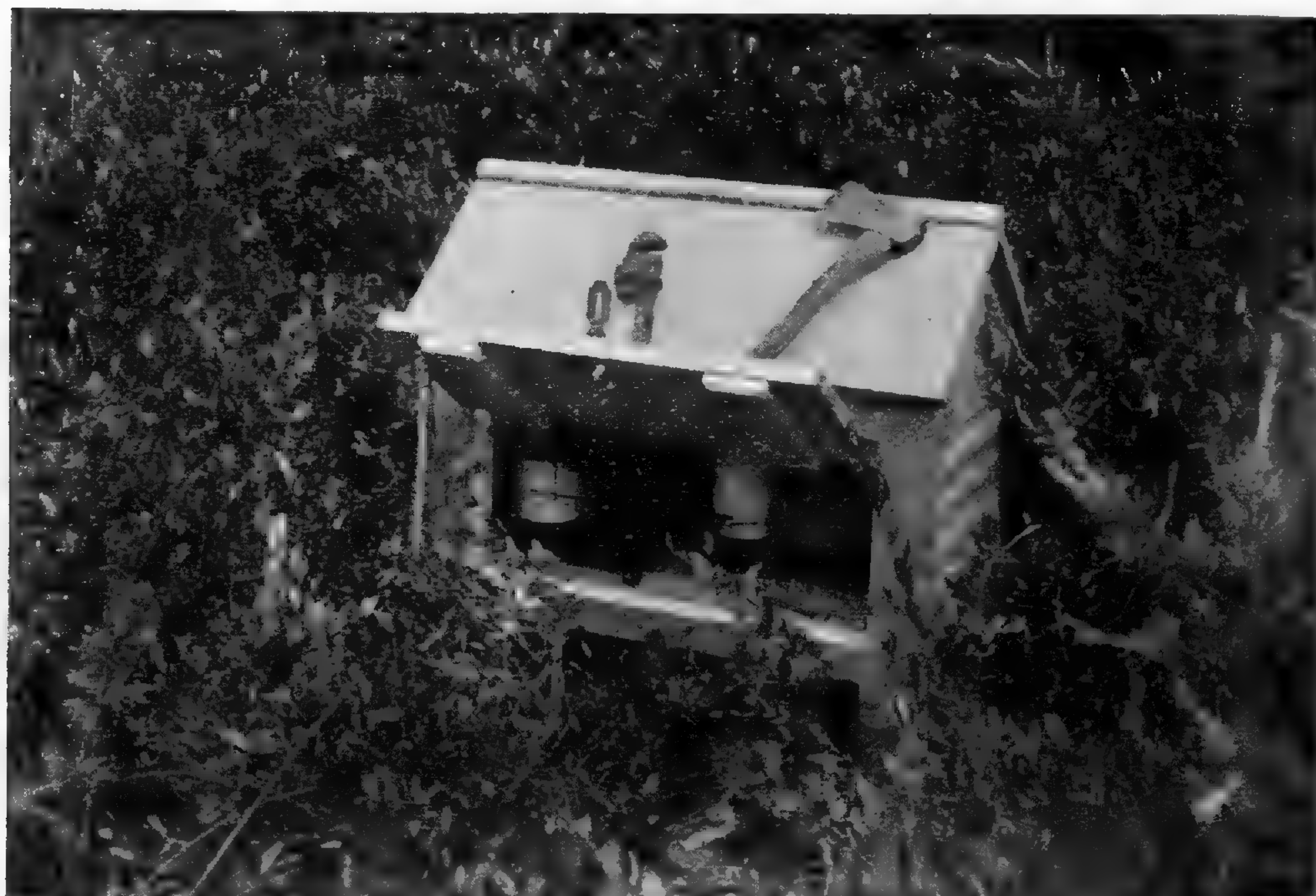
FIG. 2.—Thermographs in the bog shrub zone at First Sister Lake; the one on the left is recording air, the other soil temperature; photograph by STEELE.
