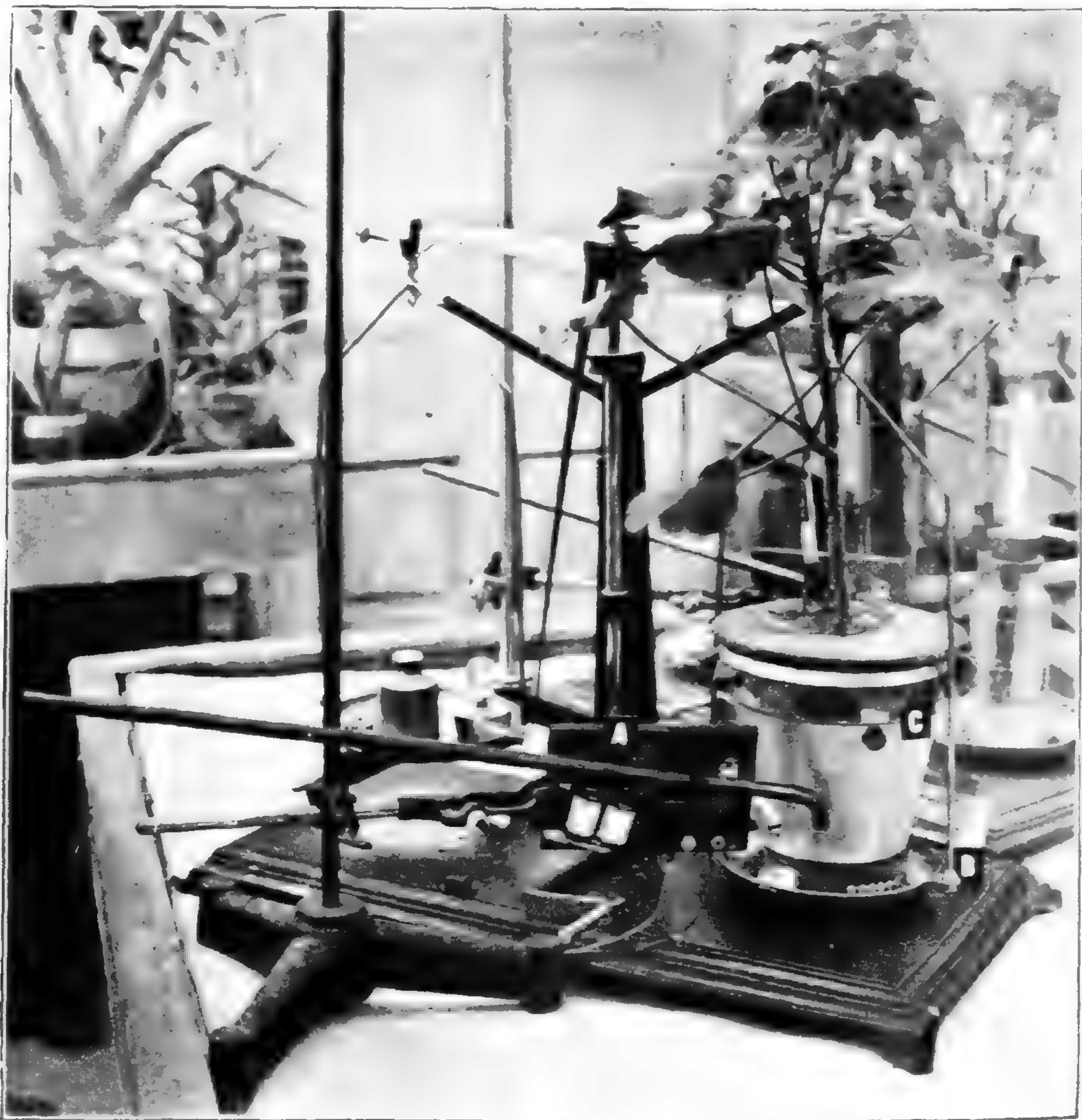
FIG. 2.—Weight dropper and circuit-closing device
