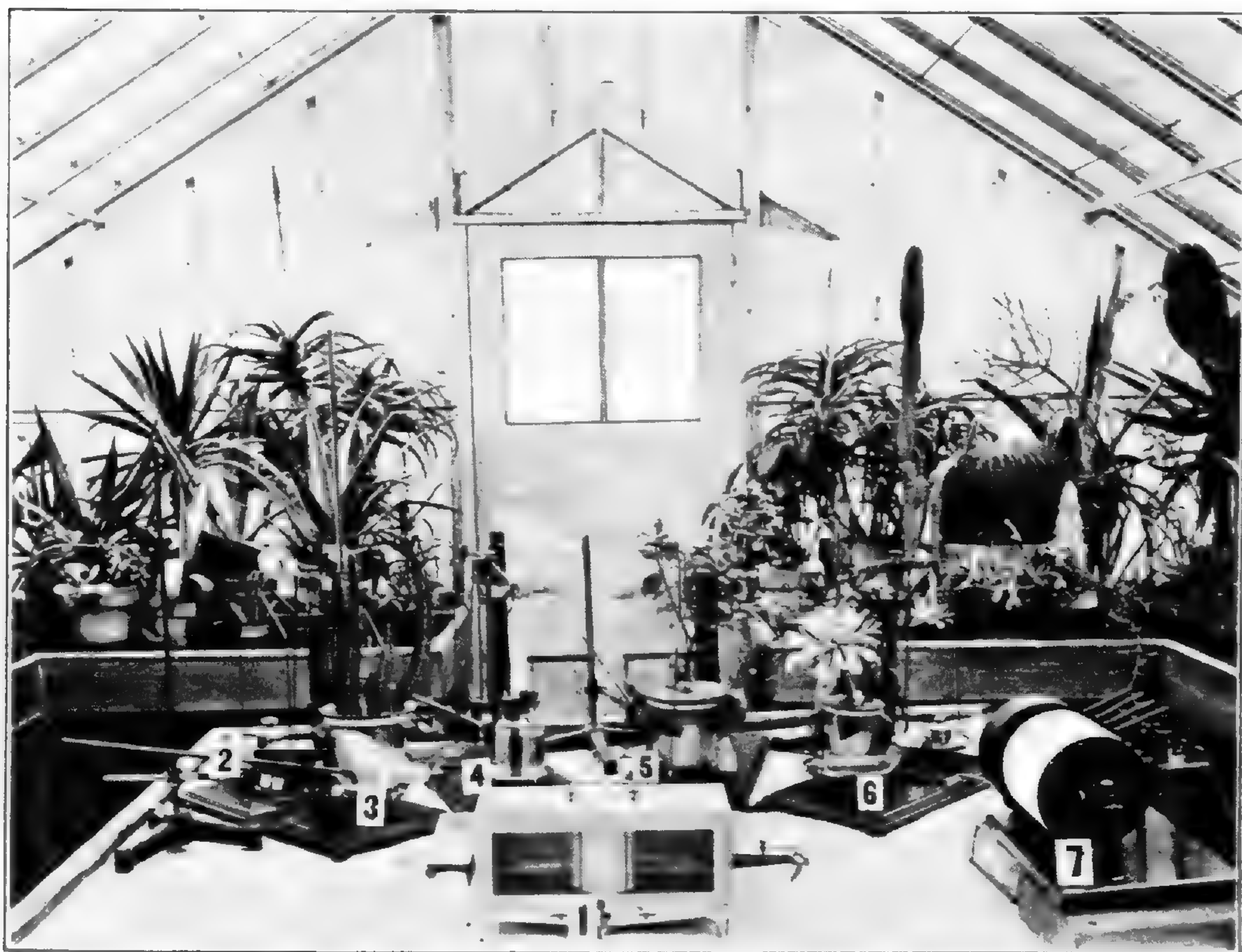
FIG. 1.—Complete apparatus for recording comparative transpiration data: 1, combined hygrograph and thermograph; 2, weight dropper; 6, irrigator; 7, chronograph.
