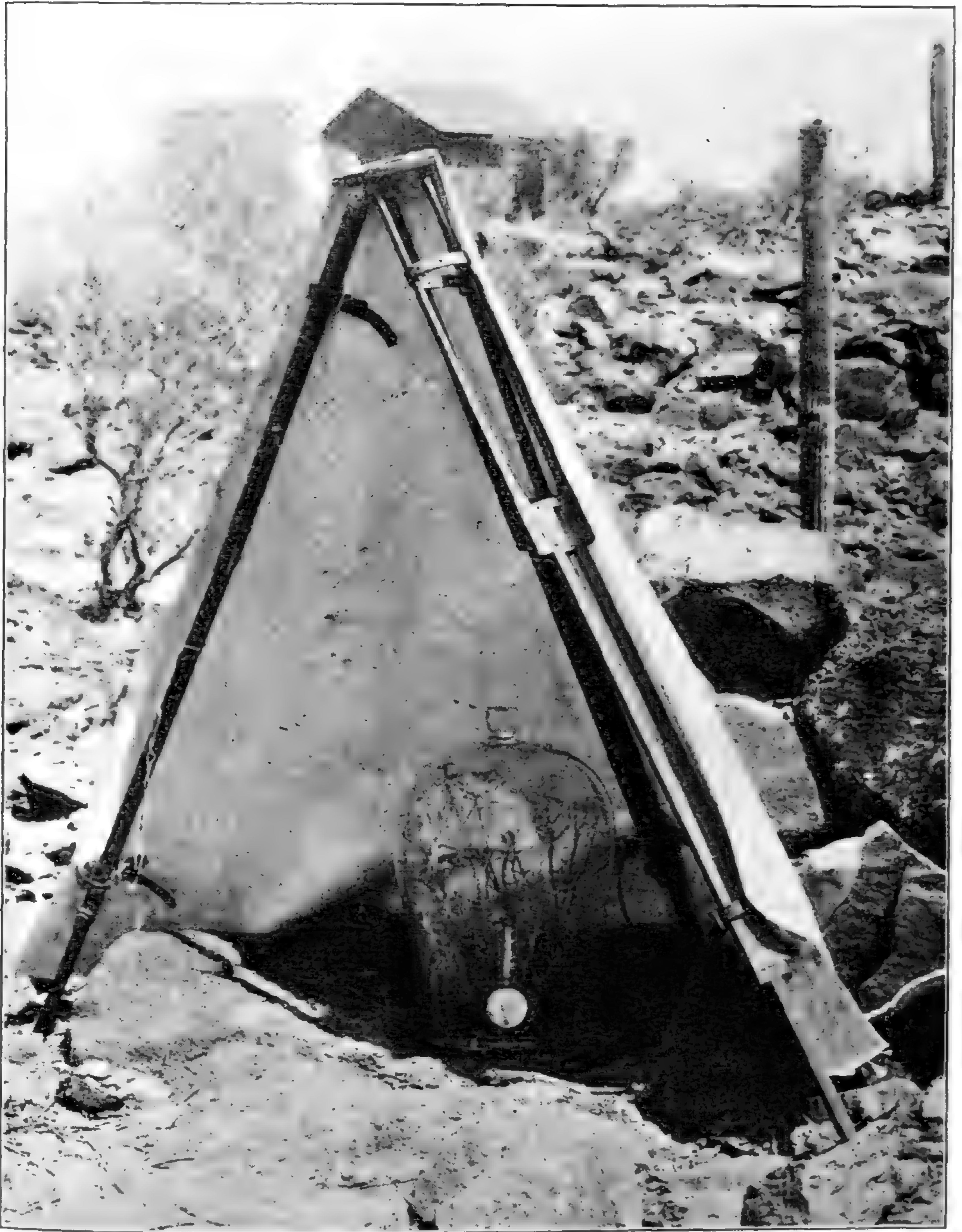
FIGURE 1. Apparatus for determining the transpiration of plants in place. The polymer method.
