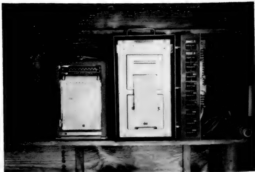
FIG. 2. From left to right the instruments are: event recorder, impulse printer, and accumulating counters. The counters registered total rainfall and wind direction.
