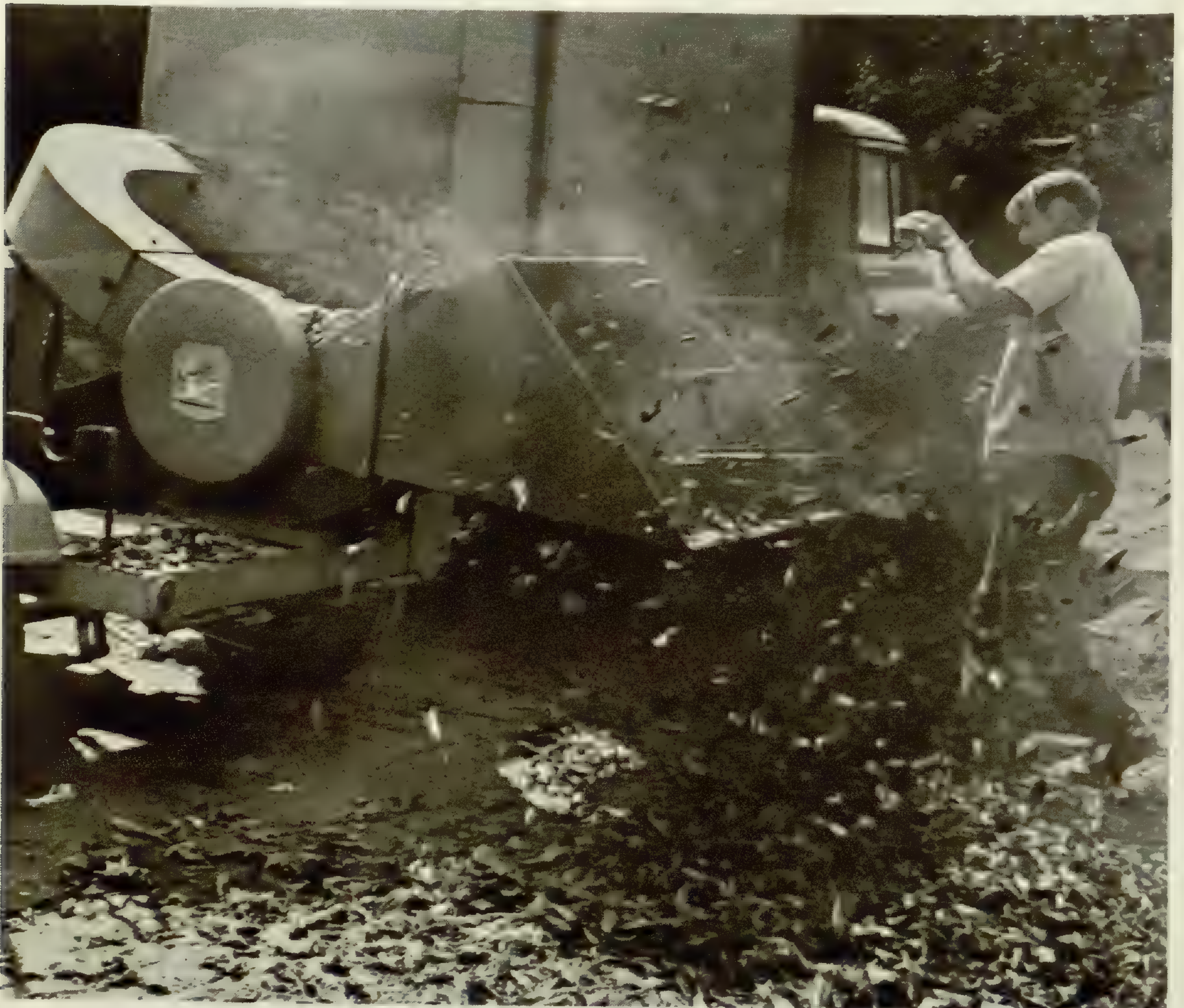
Chipper reduces tree bulk and makes drying easier. Also, disintegrates dry leaves that would interfere with the extraction process.
