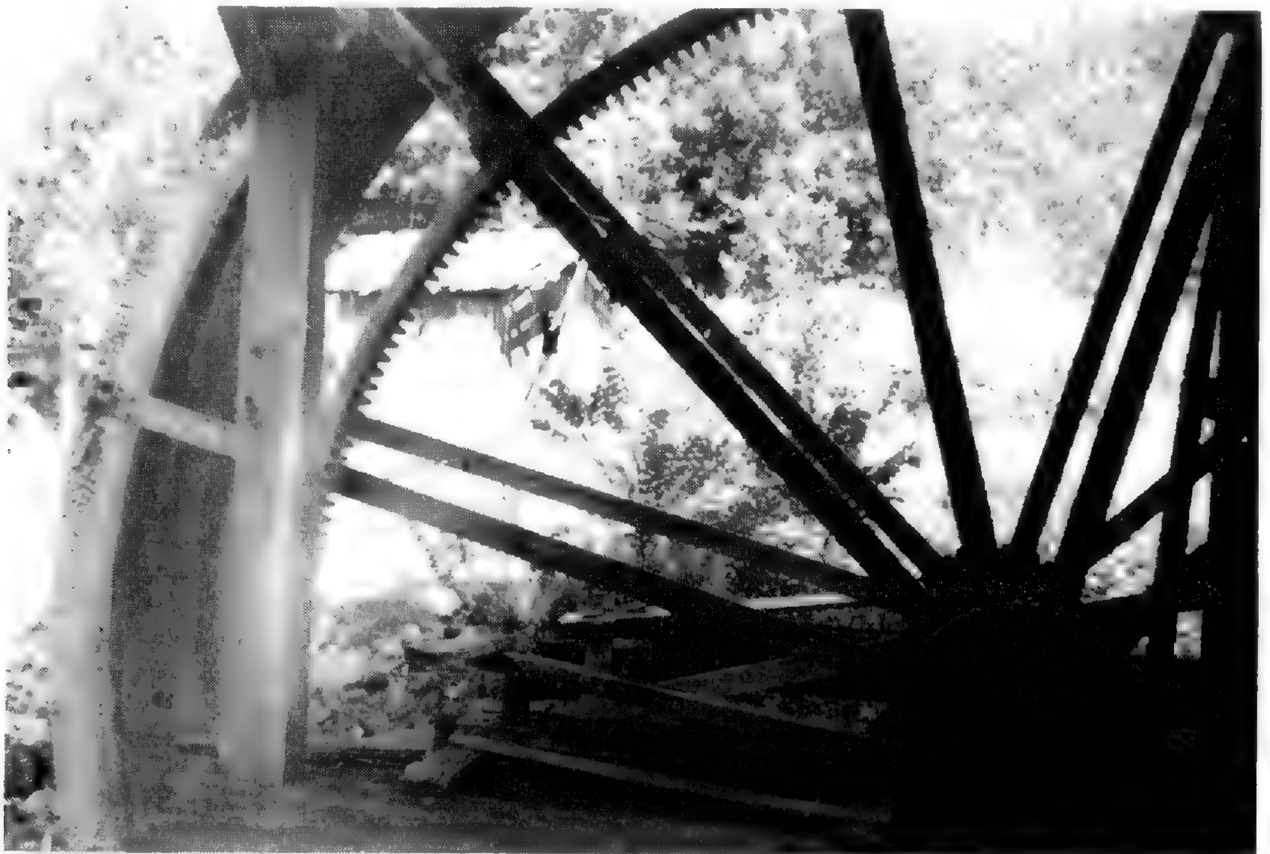
Turner's Mill, one of the largest "overshot" wheels in the Ozarks. View through the wheel from the old factory.
