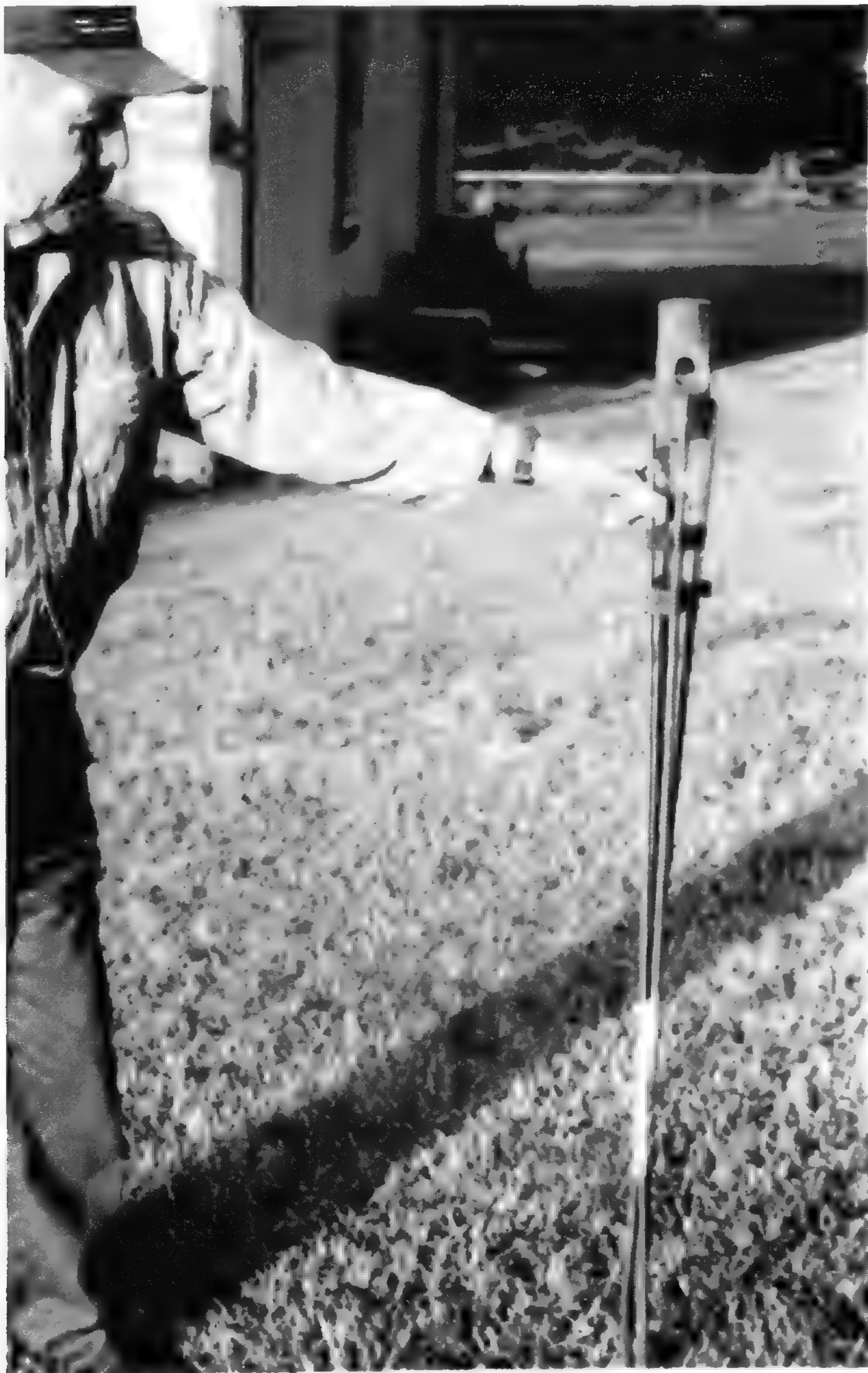
FIGURE 9.—The Carey's pestle: four rods of "rebar" (reinforcing bar) welded onto a sledgehammer head. The rods are taped together with duct tape. Mr. Carey holds the tool upside down in this photograph to display the pouncing end.
