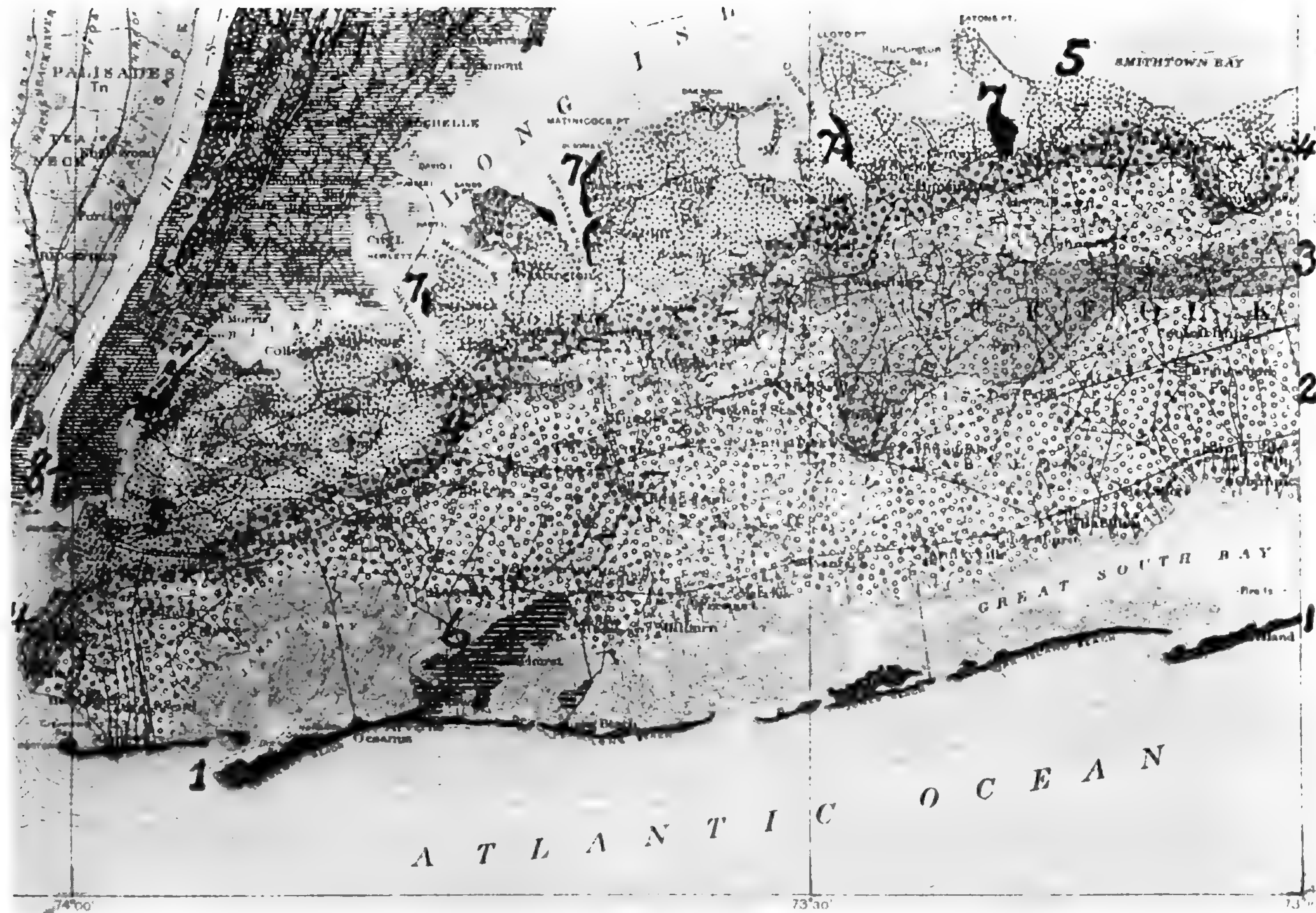
FIG. 16. Surface geology of the western half of Long Island. Pleistocene (1. Recent; 2. Overwash; 3. 1st Moraine; 4. 2d Moraine; 5. Till (or Boulder Clay); 6. Neocene; 7. Cretaceous; 8. Pre-Cambrian (Gneiss). (From N. Y. State Museum, Geological Map. Southwestern Sheet.) (6928)
