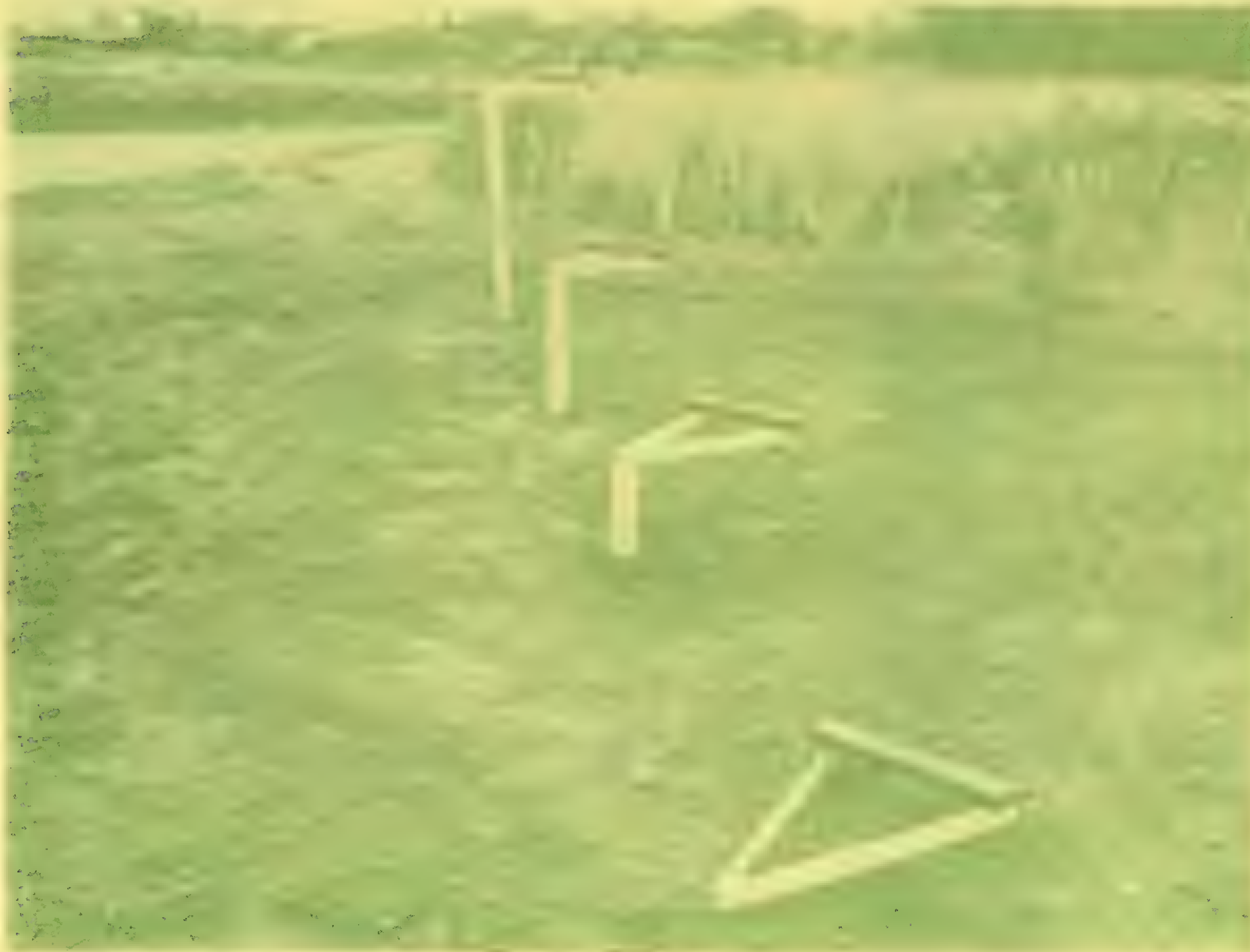
Dew gauges in position for recording the amount of dew precipitation at varying elevations above ground level
