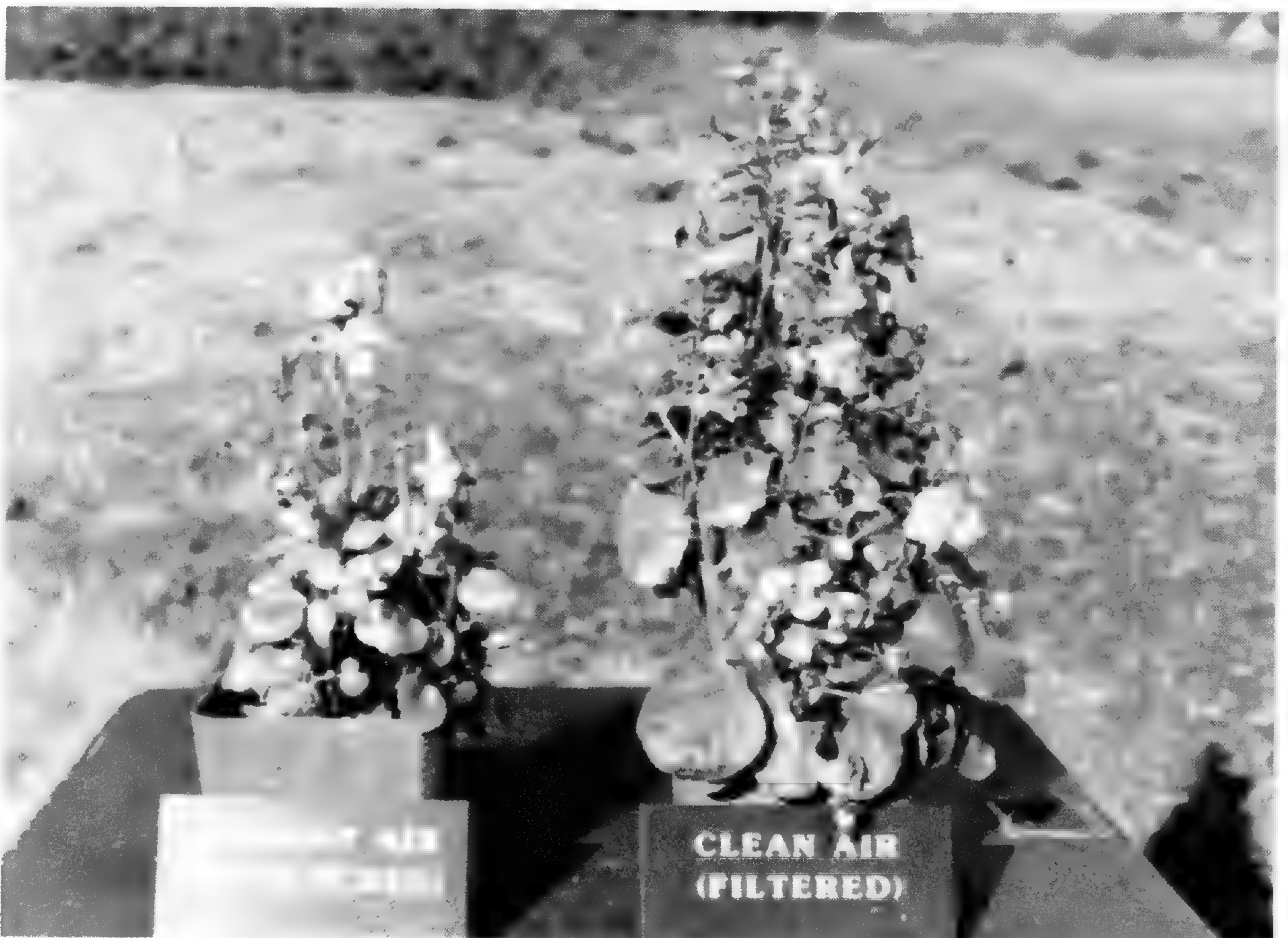
The begonia on the left grown in the unfiltered air greenhouse is one half the size of the plant grown in filtered air.
