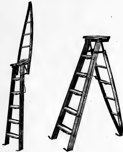
Fig. 8.—A CONVERTIBLE STEP-LADDER
