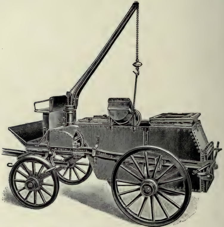
Self-dumping, Low-sided, Watertight Mud Cart used in Germany. Capacity 2.6 cu. yds.
