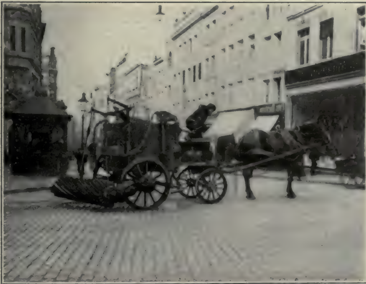
Charlottenburg, near Berlin—Watering-cart and Rubber Squeegee for Cleansing and Drying the Streets. This is a new type of apparatus which is much employed in continental cities.
