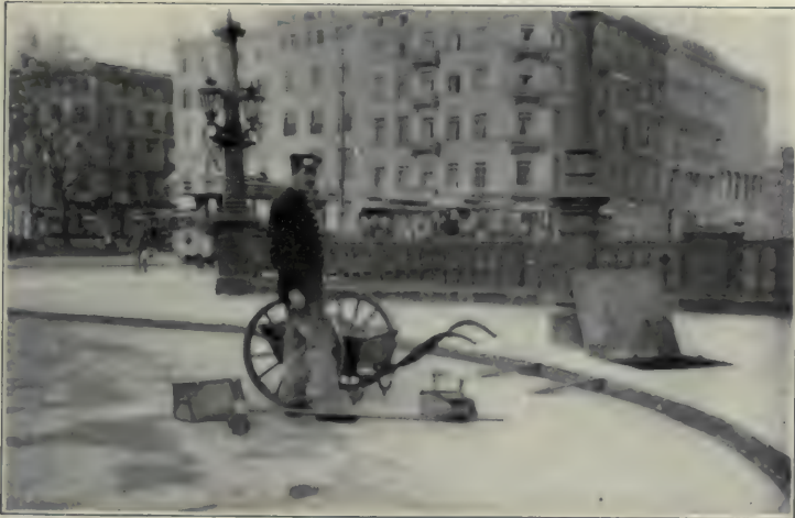
Hamburg—Street Cleaner with his Apparatus about to empty a handcart full of street sweepings into a temporary storage pit beneath the sidewalk.
