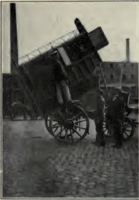
Closed Wooden Cart showing Openings with Doors to prevent Dust and method of Dumping—Cologne.
