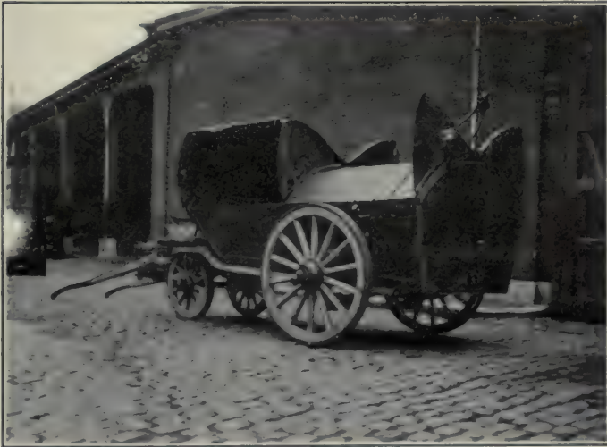
Excellent Type of Metal Dustless Dumping Cart used at Antwerp.
