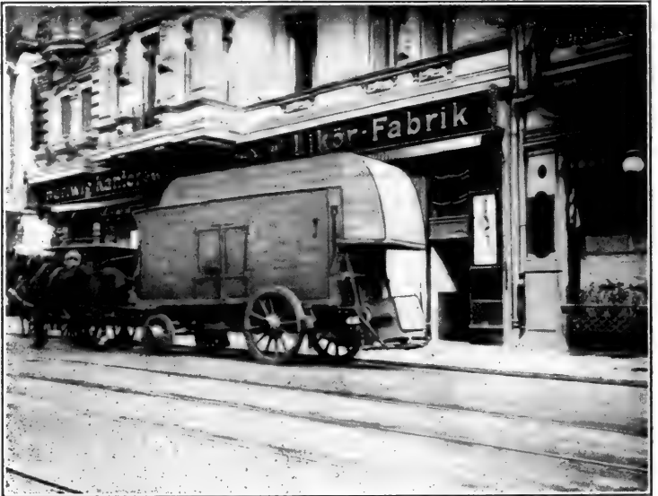
Berlin—Covered Wooden Cart used to collect House Refuse. This cart is intended to be dustless and odorless.
