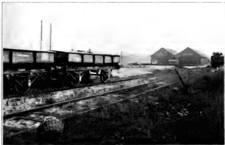
Amsterdam—Covered Metal Railway Cars for transporting Offensive Refuse to the Country without causing offense.
