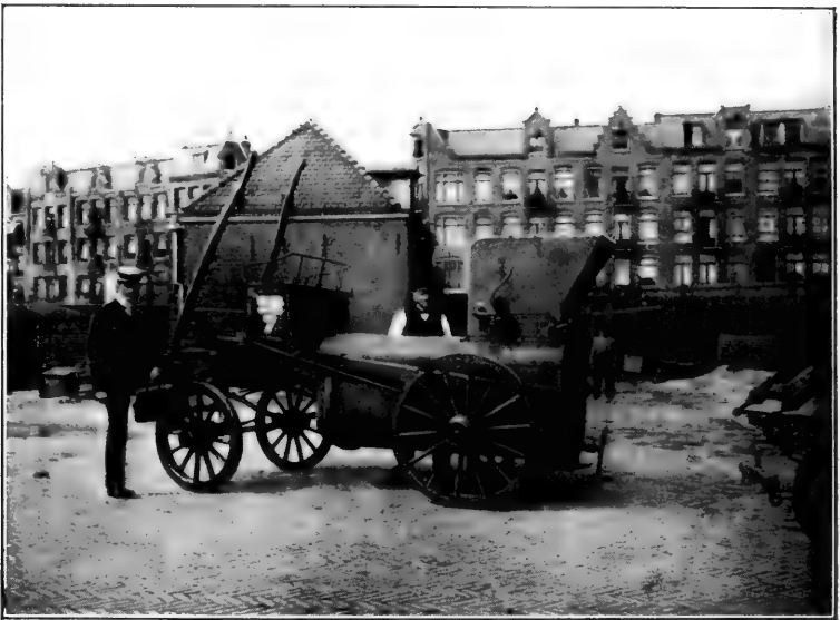
Amsterdam—Self-dumping Metal Wagon with Hood for Loading Excrement Odorlessly. An extensive nightly house-to house service is maintained.
