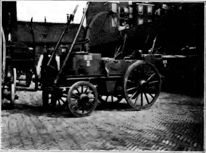
Amsterdam—Modern Type of Metal Dumping Wagon fitted with Crane for raising heavy receptacles of filth.
