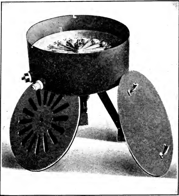
FIG. 17—ELECTRIC CENTRIFUGAL MACHINE OF LATEST DESIGN Capable of 2,200 revolutions per minute. Made by the International Instrument Co., Cambridge, Mass.
