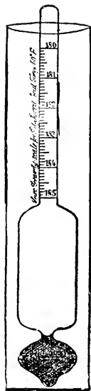
FIG. 18 HYDROMETER FOR TESTING STRENGTH OF SULPHURIC ACID
