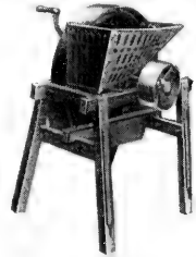
No. 832 Root Cut- ter and Pulper. Slits and Pulps.
