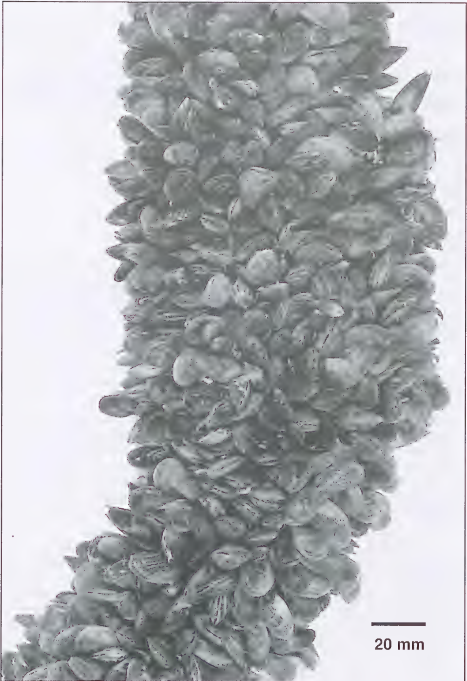
Figure 1. Section of 10 mm diameter polypropylene rope from Cullen Bay Marina heavily fouled with Mytilopsis sallei .
