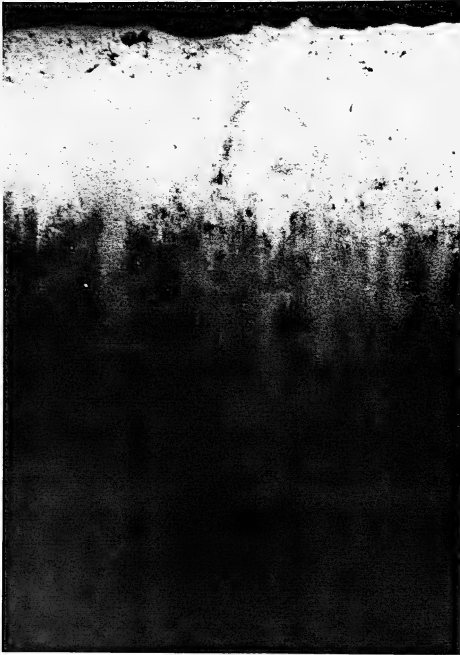
Figure 3-3. REMOTS® photograph from station E400N showing a uniform sediment-profile characteristic of ambient sediments. This is the only station sampled within WLIS showing ambient bottom conditions. Note the well-developed, relatively deep (approximately 4.0 cm) RPD boundary layer. Scale = 1x.
