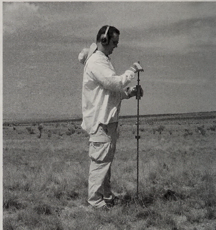
Figure 7.1. Impact penetrometer with sliding hammer elevated.
