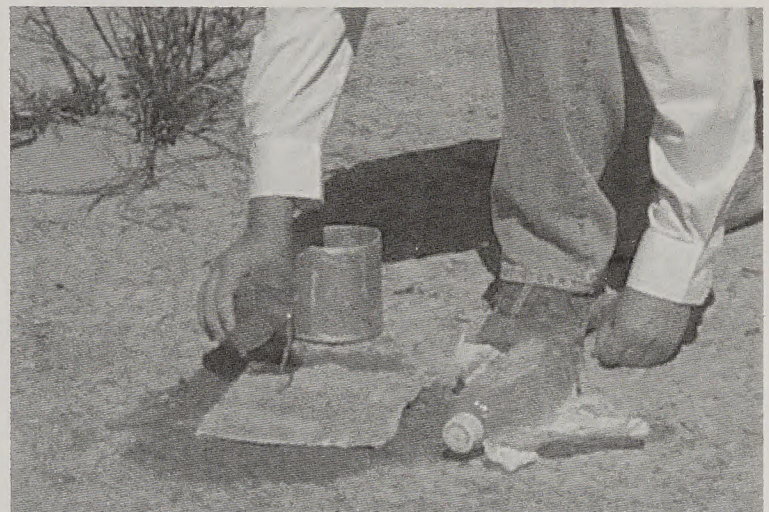
Figure 8.3. Pre-wet the soil to a 4 cm depth.
