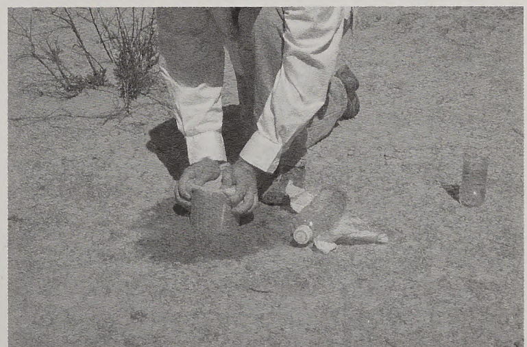
Figure 8.4. Insert infiltration ring to 3 cm.
