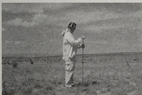
Compaction test (Ch. 7)
