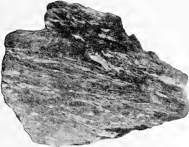
FIG. 22.—Albite schist (Hoosac schist). Dump, Central shaft. One-sixth natural size. Here the quartz lenses are more irregular and thicker; the little white specks dotting the rock are the crystals of albite.
