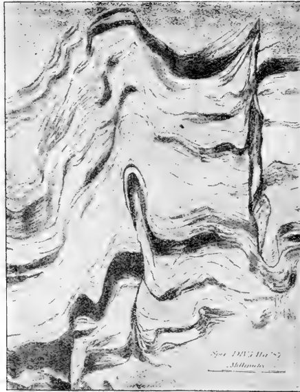
FIG. 45.—Microscopic drawing of about \frac{1}{4} inch square of a thin section of a specimen of schist from locality 741, on East mountain, enlargement 39 diameters. The light portions are mainly quartz, the dark mainly sericite and chlorite. The central plication shows the development of cleavage from a slight crinkling to a complete fault. Another cleavage plane, about \frac{1}{2} of a millimeter to the right, contains some ferruginous matter.
