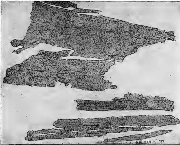
FIG. 53.—Thin section of sericite-chlorite-schist from locality 550, about one-quarter mile south of Greylock summit, enlarged 2\frac{1}{2} diameters, showing a coarse slip cleavage crossing a very minutely plicated stratification. In preparing the slide fractures occurred mainly in the direction of the cleavage, here the direction of least resistance. From a photograph.
