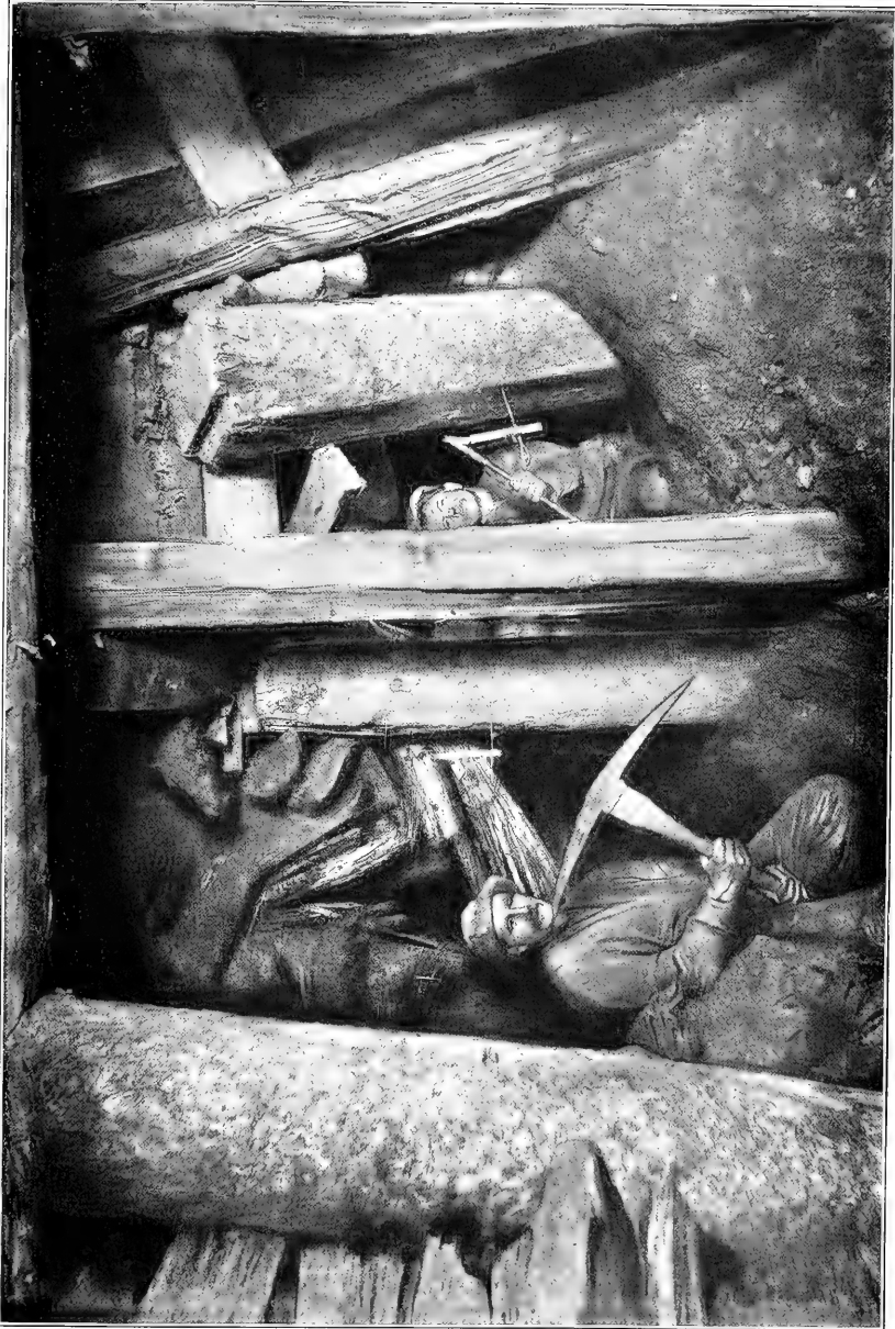
SCRAMMERS IN MINE, USING CAVING SYSTEM From photograph belonging to the Minnesota School of Mines
